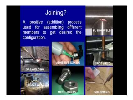
Where simpler safe components are a joint together to get the desired size and shape of the final component is called a positive process because the simpler part and the components are brought together or join together to get the desired configuration. The positive process used for assembling the different a members to get the desired configuration variety of the joining approaches can be used a.
