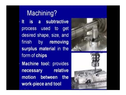
So, it is a obstructive process used to get the desired size and shape and finish by removing the surplus material. And in form of the chips you can see the one tool and the raw material is used to a to shape the material and get the desired size and shape of the components so here for the machining purpose machine tools are used. They will provide the relative motion between the work piece and the tool being used to get the desired size and shape.
