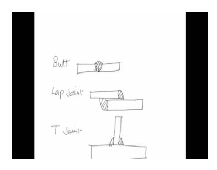
The plates to be joined or kept in overlapping position under than the weld joints is made like this near the end of the one of the plates is. So, this will be the single lap joint and if it is an both the sides then it will be the double lap joint and like t joint. In case of the t joint, one of horizontal plate is kept and now of this another member is brought vertically and then joint is made by putting in of led weld one side or in the both the sides.
