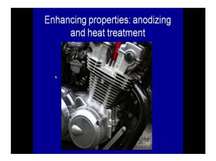
Similarly, another aspect is the enhancing properties of the components made either by the machining or welding or a forming or the costing. The life of these components is improved further by imparting the desired set of the properties. For example, the piston rings in the pistons or heat treated to improved the v r g distance and have the higher hardness. Similarly, the heat treatment of the wheels of the aluminum alloys is also carried out to increase this strength.
