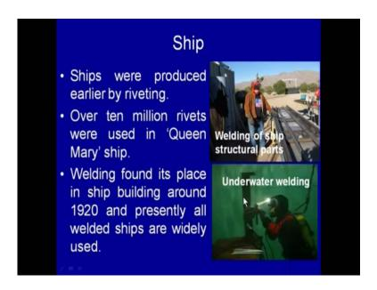
The ship are a ships were is one of the biggest industry where the welding is very extensively used for development of weld joint however earlier the ships were produced by riveting only for joining the different components over ten million rivets were used. For example, in case of the queen marry ships and the welding founds it is placing ship
