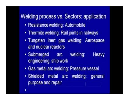
Now, the welding these used the different sectors from the application point of you the resistance welding mainly used auto metals sector of a joining then feeds. For example, car bodies and the components, that might welding is used for joining their rights in the
