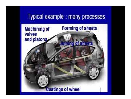
Say for example, the cars are the wheels of the car are made of the aluminum alloys which are manufactured by the casting process and the body of the car is made of the sheets which are given shape using the forming processes. The engine parts like valves and the pistons are made of the cast-irons aluminum alloys are a steels they are produced using machining processes.
