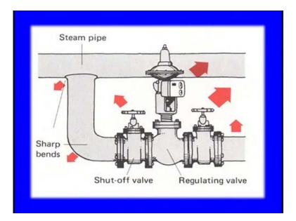
In this diagram we have the steam pipe and this is you see when it is passing through this these are some of the abrupt changes, when they are just passing through this here it has a simple this axial flow when it is just entering here. Again we have you see the you know like the band there, and these you know like the sharp bends is straight way creating some kind of the impulsive forces.
