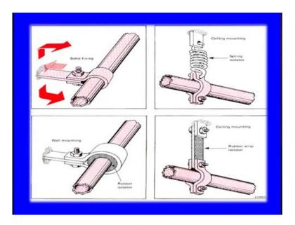
As, you can see on the in this diagram, that there are 2 main examples are given here, the first one we have you see a solid fixing is there in that, and this is straight way connected to a wall. We know that due to this action, any you know like we can say the transmission of that through this pipe there is a clear vibration is transmitted through this path.
