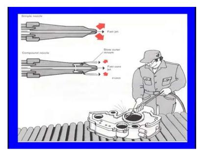
This is what you see the main action is there, when the all these you know like our engine parts are being cleaned out from this compressed air. We know that the entire this you can see the interaction the huge amount of energies are being coming out, because of the velocity the kinetic energy I can say, and the same time huge amount of vibrations are being generated, because of these impact forces.
