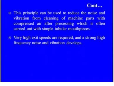
So, this is also one of the effective way of reducing the jet vibrations, you know like the jet flow and through that the vibrations are occurred, and this principle can be effectively used to reduce the vibration and the noise from cleaning of the machine part. Because, this is this has a great use we are using the jet to increase the velocity, but the same time the vibration is also increasing at the outlet part.
