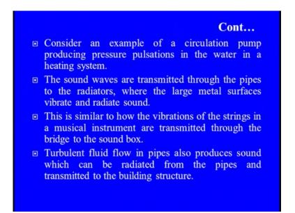
So, with these considerations of any circular pump, which is you know like producing the pressure fluctuations or any kind of you see the oscillation in the water, in any kind of heating system is a great source of the vibration or the sound generations. And these sound waves which are simply transmitting through these pipes, to the radius are; obviously, creating the huge amount of oscillation in those pipes.
