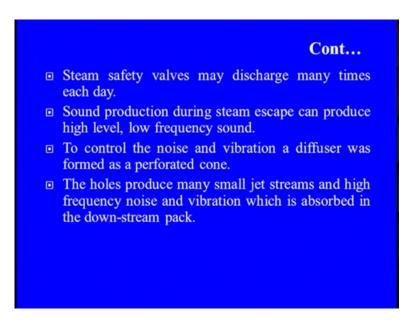
So, you see here as we have seen the steam safety valve is also you see you know like when the steam is just passing through, the safety valve is also coming under the similar kind of actions there itself. And the sound is also producing during the steam, which is escaping at the you know like which is simply producing at high level at the low frequency featured.
