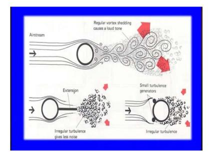
And because of this regular vertex shading, because of the vertex flow here, they are causing the clearly loud tone, and with the huge amount of energy and the air is passing from this or any fluid even rather. So, we can see that the enormous amount of energy and you see the higher vibration oscillations are there absolutely at the exit of this, and we would like to control this.
