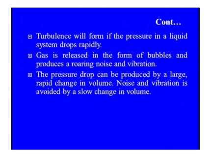
So, turbulence which is being you know like the one of the basic cause of vibration will also form if the pressure in the liquid is dropped rapidly, because when the pressure is dropping rapidly, there is a clear change in the velocities. And when the gas is released say in form of bubbles, certain you see here they are also producing the huge amount of vibrations.
