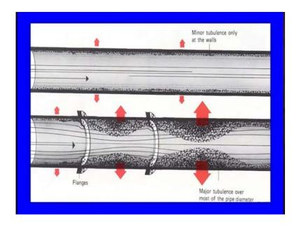
So, this is also one case in which we have a clear significant vibrations at the interaction of the fluid and solid, so like this you see here we have a clear pipe line, through which you see here you know like the flow is just passing through. And with this you see here when there is a clear you can see the first one when we have a clear fluid flow, and along the steam line no obstruction is there we can straight way say that the minor you see you know like the turbulences are there.
