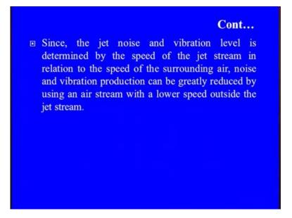
And since, the jet noise or the vibration level is determined by the speed of the jet, in relation to the speed of the surrounding air the noise and vibration production can be greatly reduced by using the air steam with the lower speed outside the jet stream. That means, you see here when we know that the jet stream is at the high velocity, it has the huge amount of kinetic energy the impulsive forces are quite significant, and because of that you see there is a clear interaction.
