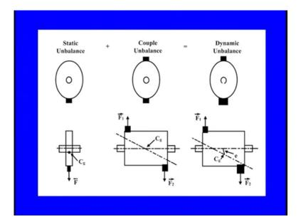
You can see on the diagram featured we have the static unbalance, in which the c g is somewhat lowered down due to the force, because of the radial force of rotor, somewhat you see it is acted towards the downward direction. And the c g is somewhat even in the microns level it is being downed, and if you are talking about the couple unbalance, you can see that this couple which is not passing through, this sharp diagonal edges.
