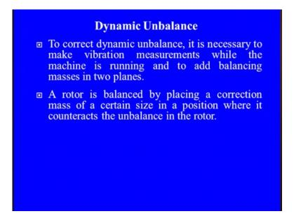
So, to correct the dynamic unbalance which is the major cause for the vibration in any rotating feature, it is necessary to make the vibration measurement, while the machine is being running. And we need to add the balancing masses into these planes in both the planes you see here, because ultimately we need to shift the c g the centre of gravity, with the centre of mass to exactly at the one point.
