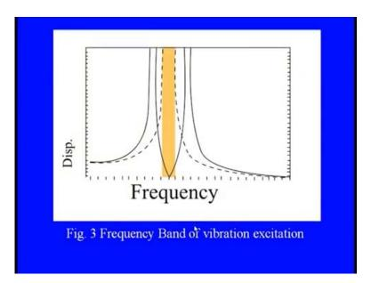
And in these cases you can see the displacement, the yellow region is clearly showing that when the system is exciting at the resonant condition, the huge amount of amplitude the energy you see that displacement feature is just infinite. But, if you want to bring it down to 0, then you see this closed curve this is what you see the closed curve, it just says that whatever the added mass the inertia block is being there.
