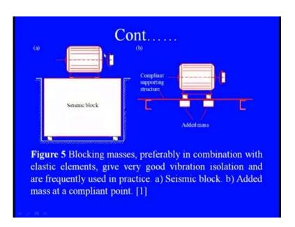
So, you see here these things are there we have a seismic block here, though you see this is a added mass on this particular entire system, which can be suppress the entire vibrations, but we need to check it out the compliant, structure support. Just like you see these added masses, and they are perfect and they can provide rather a better solution according to this space, and you see here just to absorb the vibration feature or the vibration excitation feature here. (Refer Slide Time: 43:19)
