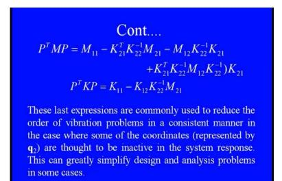
Now, you see we can simply calculate the P transpose into mass matrix into P that you see now we have a clear feature in this that it is you know like the P transpose M P is giving the variation in the mass matrix. The stiffness matrix is such a way that it is equals to M 1 1 minus K 2 1 transpose K 2 2 K 2 2 minus the inverse and M 2 1.
