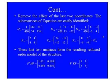
When we are now trying to remove the effect of these last two parameters, because we want to reduce this one, so what we are doing here we are simply making now the sub matrices of the equations so that we can easily identify that what are the critical parameters which can be put into the significant or insignificant criteria.
