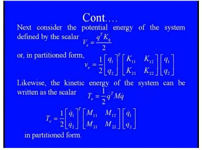
This scalar quantity V of e is nothing but equal to this, whatever the changes are there in q of t which we discussed previously that how the positioned displacement vectors are there so it is q of t into K q divided by 2. We can say that we can simply get the potential energy in form of the matrices, so this is nothing but equals to half q 1 by q 2 transpose the stiffness matrix q K q is K 1 1, K 1 2, K 2 1, and K 2 2 with the corresponding displacement q 1 and q 2.
