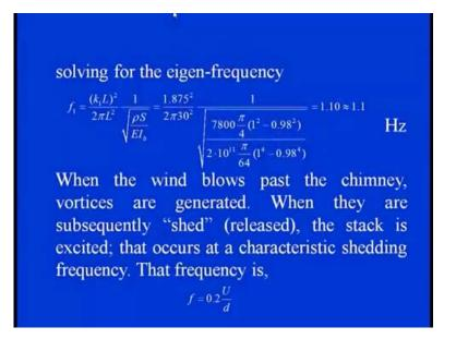
So, when we are solving this for Eigen frequency, the Eigen frequency is nothing but equals to k 1 L square divided by 2 pi L square into 1 over this, the part which we discussed, square root of rho S by E I b. E I b is nothing but equals to the modulus of rigidity for the beam and we can put entire things together you see here that, 1.875 as k L, which we calculated for the beam from the table divided by 2 pi L square is 2 pi into L is 30.
