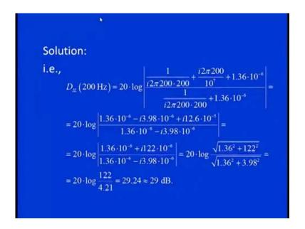
Now, our insertion loss at 200 hertz is nothing but equals 20 into log of 1 divided by 2 pi, since it is 200, so omega square, so it is 200 into 200 f square plus i omega times 2 pi f divided by 10 to the power 7. That means, you see here, we have a clear stiffness variation, so 2 this IOTA of times 2 pi as we know that, you see here which we
