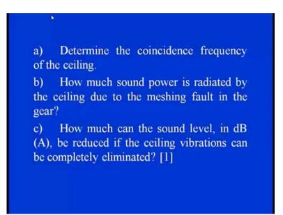
Now, the first thing we would like to find out, the coincidence frequency of the ceiling, because of the machine excitation. Second the power, the sound power which is being radiated due to the meshing fault, because we have now the exciting frequency then how much power is being radiated through this ceiling. And you see here, because and it is
