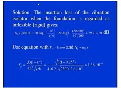
So, as we know that, the insertion losses of the vibration isolator can be straightaway calculate when the foundation is solid, is nothing but equals to 20 log 1 minus omega square divided by k by m, where we can calculate the omega as the exciting frequencies when we know that, 2 pi f square. And the stiffness is given to us, the mass is given to us, so for 200 Hertz say, now we are going towards the higher mode of this excitation.
