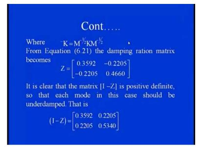
And then when we are putting this matrix to the main equation of K, which is nothing but equals to M inverse half K M inverse half or even M inverse minus M minus 1 K M 1. So, it is what you see the balanced equation, which we discussed in the last chapter of that. So, the damping matrix ratio, whatever you see the damping ratios are there in the matrix form, it is nothing but equals to 0.35 minus 0.22 minus 0.22, that is what the symmetricity and 0.466.
