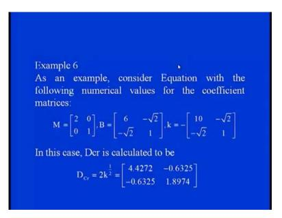
So, critical damping is nothing but equals to D critical equals to 2 k to the power half, so we can say that, this matrix is nothing but equals to we can simply square root of this stiffness matrices. So, we have 4.42 minus 0.63 minus 0.63 and 1.8, so this is what my critical damping matrix.
