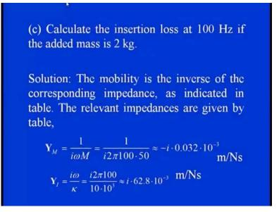
So, now you see here, the first case was this, the second was the mobility replacement in the total and the third case is that, the insertion losses at 100 Hertz frequency if the added mass is 2 kilogram. So, how much you see the insertion losses are there at that exciting frequency. So, the first case, the mobility is nothing but the inverse case of the impendence, as we know that. So, we can calculate the impedance Y M, the impedance equals to 1 by i omega m.
