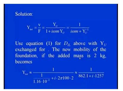
So, now, you see we can straightaway calculate Y U equals to v by F, where it is the Y total we would like to calculate. So, it is Y U v divided by I 1 plus i omega m Y U or else you see here, when we are just dividing these things, it is equals to 1 divided by i omega m plus Y to the power minus 1. So, you see here, the insertion losses for that can be straightaway exchanged when you see, when you are just exchanging Y U with the added mass.
