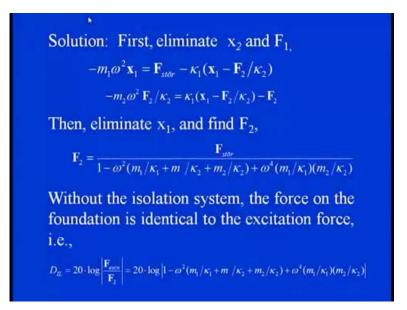
And when we are trying to eliminate the X 2 and F 1 then we have minus m 1 omega square X 1 equals to the F, whatever the storage feature minus k 1 into X 1 minus F 2 by k 2. And when we are just making balance of these things, we have minus m 2 omega square F 2 by k 2 equals to k 1 into X 1 minus F 2, which is the excitation force at the foundation divided by k 2 minus F 2, this is what it is you see here, we are trying to modify the equation based on the elimination of X 2 and F 1.
