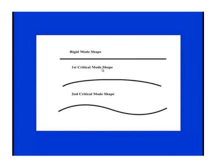
All these feature are all these features are being featured out, when the rotor is rotating at the different critical speeds. So, you can see that the first critical speed, we have a different you see in the entire shape is like that. So, we need to adopt a different kind of methodology. When we are on the second critical shape you see here. We have a wave feature and a different corrections are to be needed there itself.
