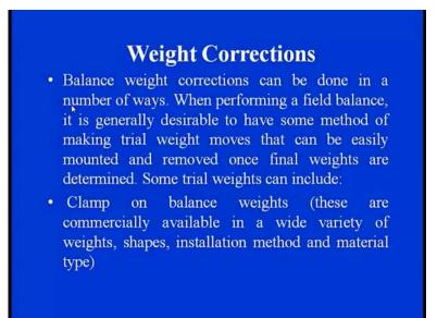
Like clamp on the balanced weight sometimes we are saying that you see the wide variety of weights. Even the weight we need to check it out what exactly the level of the weights. In terms of masses, the shapes, the installation methods, and second is the material because sometimes when we are adding the weight they are also providing some kind of material damping according to the material type.
