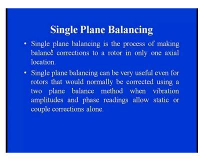
So, the first category in the balancing is the single plane balancing. And this is the process of making balancing correction to the rotor just with the consideration of one
