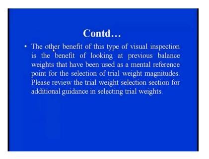
So, the other benefit of this type of visual inspection, is just giving that what the previous weight situations are, so that the selection of the trial weights can be appropriately chosen. To just check it out to see the balancing features in that.
