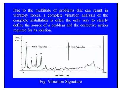
Even we can find out the, any kind of inadequate base or flexible foundation or even we can find out that, what is the resonance of the machine or any component so that, you see here we can evaluate that. The distortion can be also you see, you know like, in the field due to service conditions or anything you see, the design parameters, in the piping part and improper design for any component, can raise the vibrations in that. So, we can see
