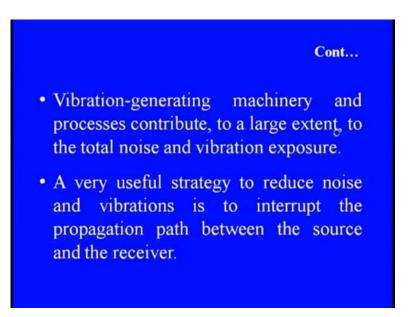
So, vibration generating machinery and the processes, they are both contributing to the maximum extent not only to the vibration exposure, but also the noise which is coming out from the devices. So, a very useful strategy to reduce the noise and the vibration is to interrupt, the propagation path between the source and receiver which we already discussed about that.
