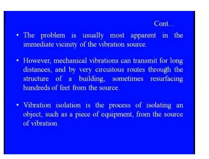
So, the problem is usually most apparent in immediately vicinity of the vibration source, and we need to apply straightway, the concept of vibration isolation on these sources. However, mechanical vibration can transmit for long distances as well, and by very continuous rotors or the routes with this, where you see you know like the rotating elements are there.
