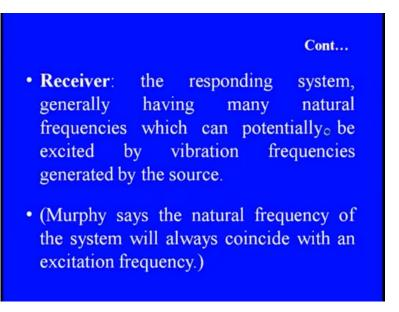
And the receiver is something, which is you know like the responding system generally having many natural frequency, which can potentially be excited by vibration frequencies which are generated by the source. So, the natural frequency you know like is being defined sometimes, you know like by the murphy, and it says that it will always be coincide with the exciting frequency, and you see here, you have always a huge amount of energy at the time of this exciting frequency.
