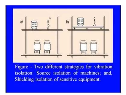
The a part, and b part; these two different strategies are showing for vibration isolation, first the source isolation of the machine, and second the shielding about the sensitive equipment.
