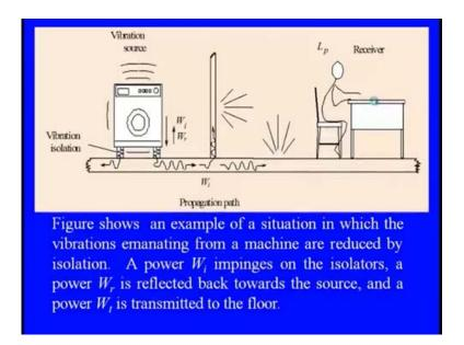
As, we can see you see here in this diagram, the source is something which is you know like the rotating machine, and it is creating huge vibration along with the noise. We can see that the vibration isolators are being straightway provided in between the vibration source, that is machine to foundation. And say that you see here you know like the controller or anyone who are any person is working near to these places, they have a clear exposure of these things and we want to reduce that.
