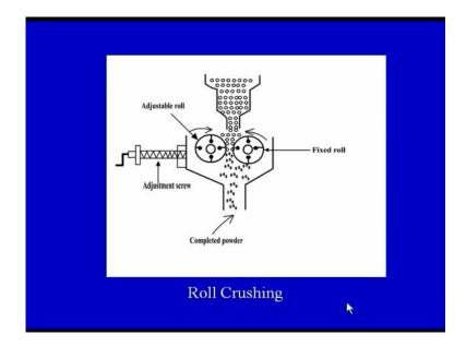
So, in this particular diagram we can see that this is a ceramic raw material hopper through which the bigger particles are coming, they are crushed inside the two rotating rollers and finally we have getting the completed powder or the crushed powder or very fine powder. So, there are these two roller and this is the adjustable roller, it is written clearly adjustable roll. This is the adjustable roll and this is the fixed roll.
