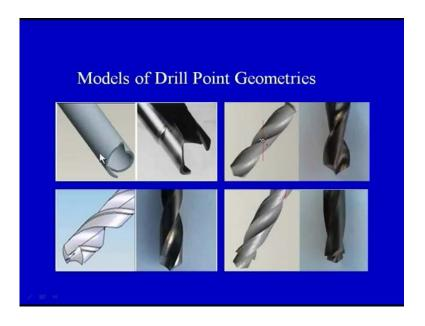
So, here you can see the models of the various drill point geometries there are this is the model; which can be modeled in any geometrical model ling software, this is one model and this is the tree panning tool and this is the actual tree panning tool this is you can see
