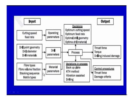
So, my material parameters are fixed fiber type is glass, fiber volume fraction suppose 60 percent, stacking sequence is normal all layers are made up of glass fiber only and the matrix is epoxy. So, glass fiber reinforced epoxy matrix one material; drill point geometry suppose, simple twist drill, drill diameter suppose 8 millimeters, drill materials suppose high speed steel. And, cutting speed and feed suppose I fix a range that cutting
