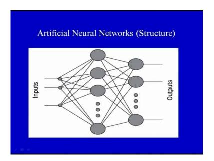
So, this is an artificial neural network. So, in artificial neural network; we can see there are set inputs 1, 2 and 3; there can be other inputs as well more inputs can be used and we get the output. So, this is the intelligence that is inbuilt. So, this is the intelligence that developed by giving a set of input data that data has to be huge that has to be have a wide range. So that the network gets trained better and once the network gets trained better
