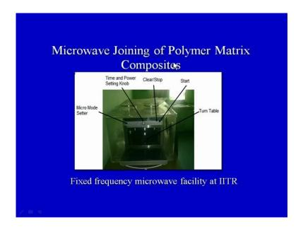
This is a typical microwave joining of polymer matrix composite on your screen, you can see there is a time and power setting knob time and power setting knob in which we can fix the exposure time, and the power, as we have seen that in the previous slide the power can be 900 to a maximum of 900 watt there can be other high end microwave ovens where the power powers can be even higher, but we can set the power according to the requirement.
