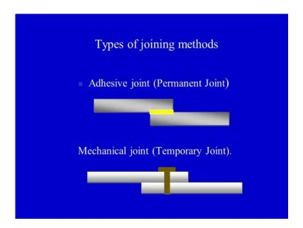
On your screen, you can see the two mostly used joining techniques or types of joining methods. So, first one is the adhesive joint which is a permanent joint means, the two composite adherents, when they have joined been joined together they cannot be dis assembled without breaking the joint. So, adhesive joint is a permanent joint on your screen, you can see this is one adherent this is another adherent; and this yellow portion
