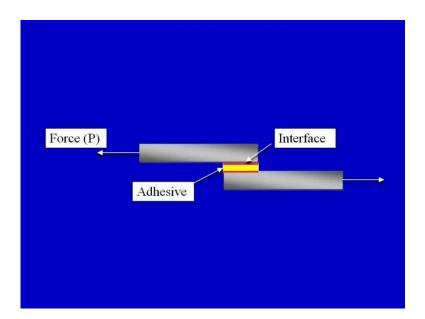
So, on your screen whatever we have discussed I will just once again revised, this is the adherend composite adherend, it can be made up of glass fiber reinforced plastic or carbon fiber reinforced plastic another adherend, which can be of the same material like
