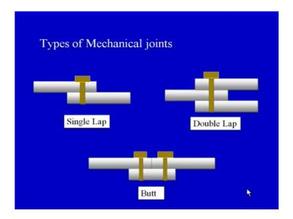
Then we have the types of mechanical joints, we can have again a single lap joint, which is shown here a double lap joint. On your screen, you can see and then a butt, butt joint is also there. So, we can make different types of joints in case mechanical joints also.
