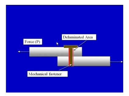
Now, on your screen what we have already discussed, these are two composite adherends adherend number one adherend number two, and the loading has been applies in between we have a mechanical fastener. And we can see this is exact type of delaminated area why this delamination in the adherends has taken place, because of the hole making
