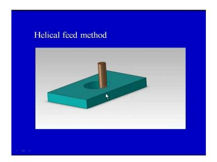
So, we can see the helical feed method this is the drill point geometry and this is the composite laminate in which the hole is being generated. So, the drill would moved on helically and it would certainly lead to certain advantages which are not possible with the conventional drilling method.
