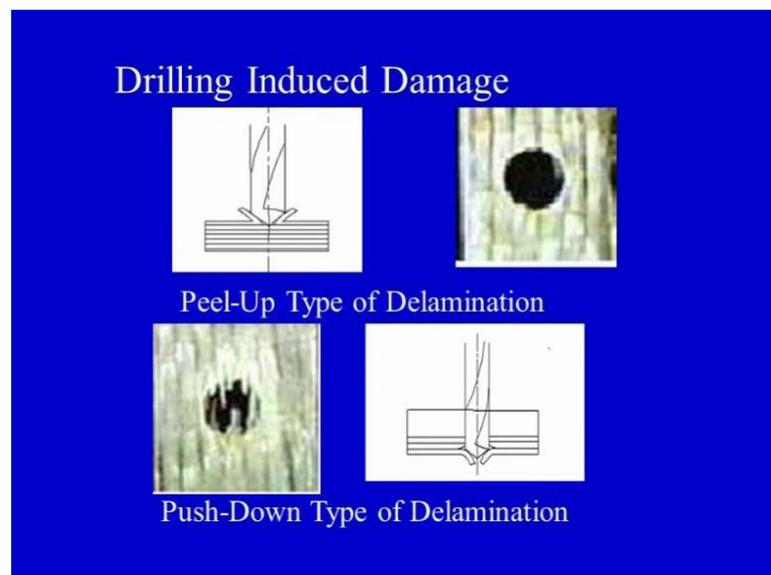
Now, this particular diagram on your screen shows the drilling induce damage. Now our focus is on the drilling operation in the polymer matrix composites. So, on your screen, you can see this is the damage that is called peel up type of delamination. This has this
