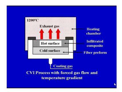
So, this is the diagram on your screen you can see, we have a heating chamber this is the heating chamber in totality 1200 degree centigrade, which is one of we can say range of temperature, it can range may be 1100 to 1400. So, general temperature is mentioned that is 1200 degree centigrade depending upon the different types of composites, we may require to change the temperature. So, basically we have a heated chamber.
