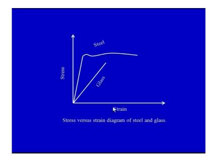
Where, so here we can see that there is no abrupt failure in case of steel. There can be necking that may take place, may be the steel will elongate the cross sectional area will slightly reduce. When we are applying the tensile load after, we can say some passage of time, the final catastrophic failure or a final abrupt failure would take place. But before the failure certain amount of deformation would be noted. So, the strain would be there that is change in length to a original length.
