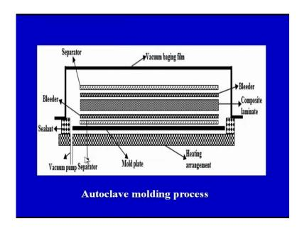
On your screen, you can see the diagram we have a mold plate this black potion on your screen this is the mold plate these are the 2, you can say bleeder this is one bleeder this is another bleeder and then there the separators, this is the separators and this is the composites.
