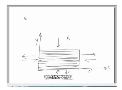
So, on your screen, you can see just try to understand that, suppose this is a simple composite part and we have all the fibers in one particular direction. Now, suppose we have and I blow up this particular area if I look it from this side. I have the fibers ends like this. So, these are the fiber ends and in between we have got the matrix material. The dark portion is the matrix material and we have a fiber ends.
