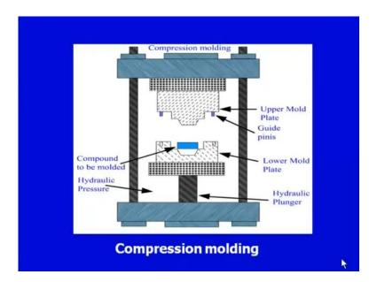
Now, you have a diagram a very simple diagram on your screen. You can see in the diagram you have a upper half mold and you have a lower mold half, this is the lower mold half and this is the upper mold half. You can see, when this mold halve of would
