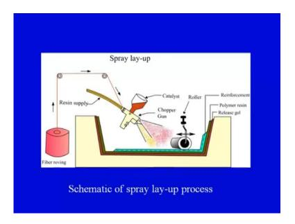
This is the photograph that we have seen in the last lecture, also this is the spray lay-up process. Again just to revise I will highlight the important aspects, there is a fibrous reinforcement and there is a resin supply with the, in the form of this tube, there is a catalyst or the hardener so resin hardener and fiber are getting mixed in this spray gun or the chopper gun and the mixture is getting sprayed on to the mold surface. This yellow colored component you can say this is the mold.
