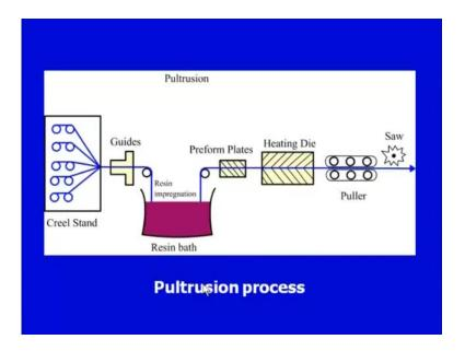
Now, this is a simplest diagram of the pultrusion process, you can see these are the fiber creels this circular portions this you can say this can be called as the this in totality can be called as creel stand. In this creel stand there are different creels and from these creels the fibers are coming. So, usually the diameter of the fiber is very less suppose in case of glass fiber the diameter of the individual fiber may be ten microns may be eight micron
