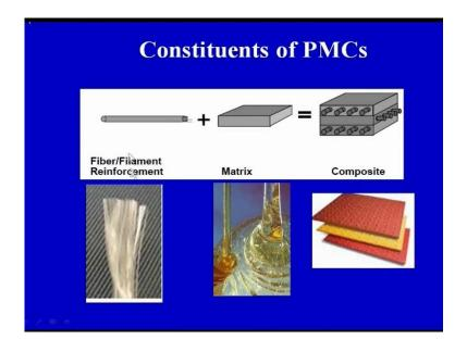
As you can see on your screen, you have the fibers and the matrix. So, fibers and the matrix, they add up to make this particular composite which we have just I have drawn one diagram of a composite laminate. In that laminate, there are fibers in this particular form and there is a matrix in you can say semi liquid form, in a semi solid form. And when these two things are combined together we get a composite plate. So, here you can see different types of coloured composite plates.
