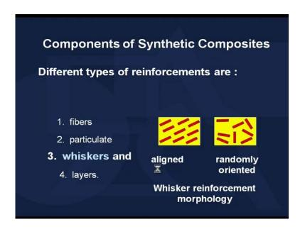
Also the reinforcement can be in terms of whiskers, in this particular slide you can see the reinforcement is in the terms of whiskers. So, all the whiskers are aligned in one direction here and they can be randomly oriented whiskers in this slide also the yellow portion shows the matrix and the red portion shows the whiskers or the reinforcement those reinforcement can be aligned in a particular direction depending upon the specific requirement of the part or it can be randomly oriented.
