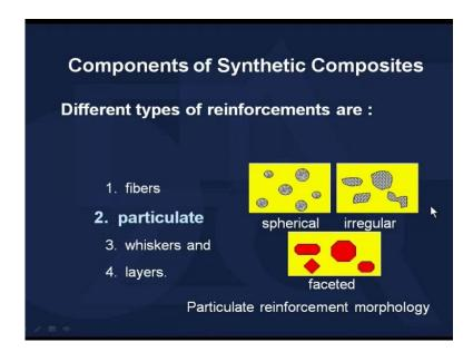
Then in another case, we can have the reinforcement in terms of particulates in this particular slide you can see the matrix is being representing by the yellow portion and the
