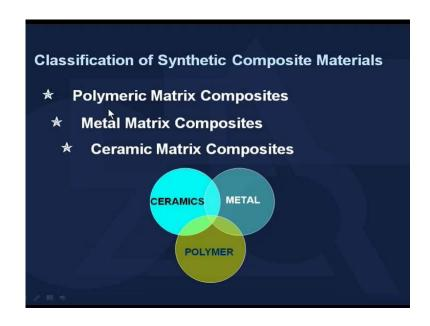
So, broadly we can classify the synthetic composite materials into three categories. So, that is polymeric matrix composites, metal matrix composites and ceramic matrix composites. So, you can see ceramics metals and polymers. So, these three types of composites are broadly used and in our series of lectures we would be focusing primarily on polymer matrix composites and metal matrix composites.
