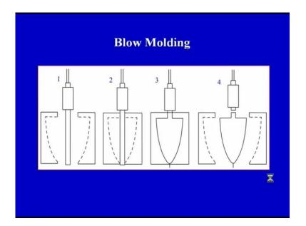
So, let us know see and try to understand the four steps involved in the blow molding. As I have already drawn one diagram to explain the basics of blow molding. Let us again see this is the parison or the heated plastic raw material. You can see the arrow is
