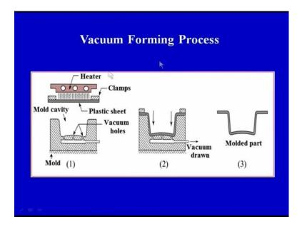
Let us see now the vacuum forming process we have the heater that is the heating arrangement. We have the two clamps to fix the mold fix the sheet that is the plastic sheet, this is my plastic sheet. So, this fixed with the help of clamps heating arrangement is there this, these two clamps sheet would be placed here after the sheet has soften. Finally, we will apply vacuum here and once the vacuum is applied the sheet would conform to the shape of the mold.
