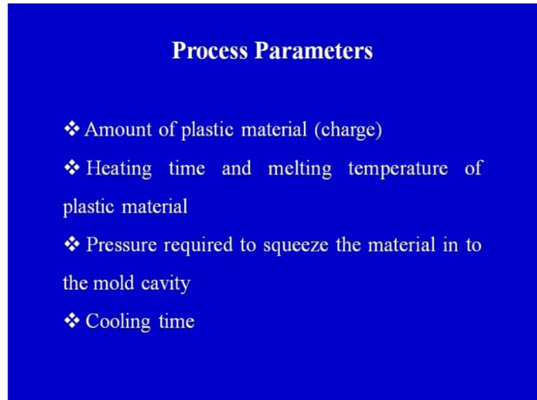
Now, what are the important process parameters in compression molding? Now let us see the amount of plastic material that how much plastic material we should keep in the lower fixed mold half that is important that has to be decided. Second is the heating time and melting temperature of the plastic material for how long we should heat the charge that is placed on the lower fixed mold half, and what is the melting temperature of the raw material that has to be taken into account.
