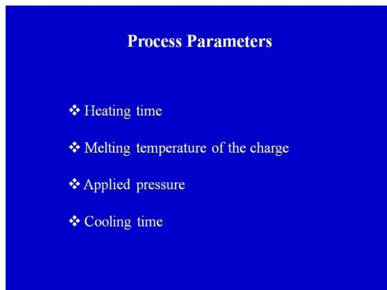
So, on your screen, you can see that what are the important process parameters that are very very relevant in case of the transfer molding process. So, first is the heating time. If you remember around the heating pot there were so many heating element. So, how much heating time should be there and for how long the polymer charge that is there in the transfer pot should be kept under the heated condition that is one process parameter.
