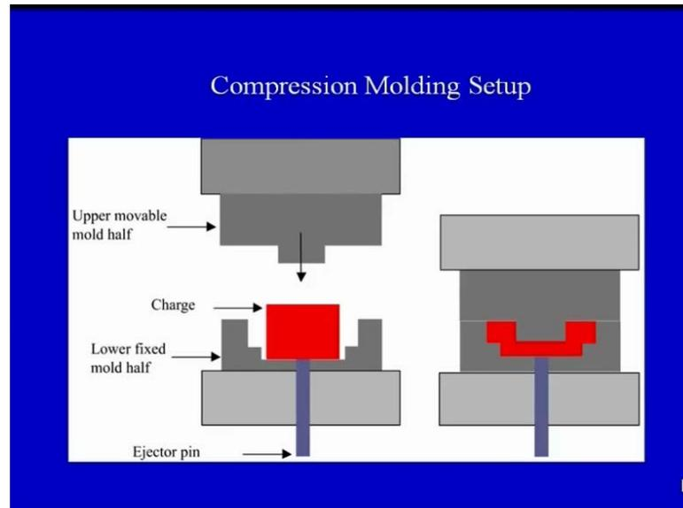
This is a simple diagram which I have drawn this is the compression molding process. So, we have the upper movable mold half this is moveable this is moving in this direction. We have a lower fixed mold half this is the lower fixed mold half this is the charge red color this is the polymer which we want to give the final shape. Now, this what I have not mentioned in the diagram that I have drawn this is the ejector pin, now this particular ejector pin can be used to eject the final product.
