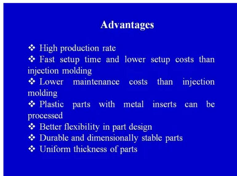
Now, what are the advantages? The advantages are very well mentioned on your screen you can have an idea, first is high production rate. So, the production rate is high in case of transfer molding. It can be automated also, automated process can further improve the
