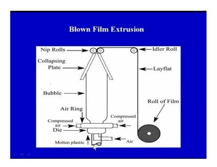
In this particular diagram, we can see that we have a molten plastic coming out in the vertical fashion like this. The air is entering from here this is the die vertical die, with circular cross section molten plastic is entering the die. The air is blown out the molten plastic, this is the air ring compressed air is entering from here and from this side also. This is the bubble, which we are talking about this is the bubble, which is formed and this is pulled up with the help of this nip rolls.
