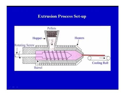
We can see, let us first see what are the important elements in this diagram? We have the heaters these are the heating arrangements or the heating elements all around the periphery of the barrel. These are the heating arrangement, this is the barrel. Hashed portion is the barrel and then this is the rotating screw, the direction of rotation is also shown. It is marked by an arrow rotating screw this is the rotating screw.
