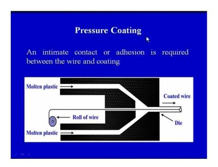
In a different case that is pressure coating, we can see an intimate contact or adhesion is required between the wire and coating, why? Because the coating is taking place within the setup only. The roll of, from the roll of wire the wire is coming. If you see this is the movement of wire wire is coming from this direction it is moving in this direction.
