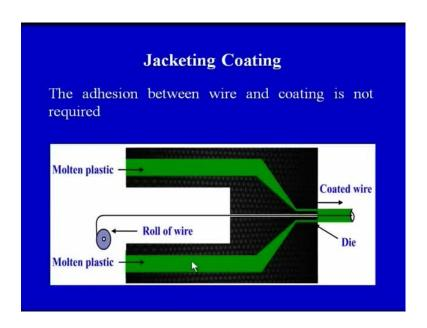
So, this is the process of blown film extrusion then we have a jacketing coating in which we see the adhesion between the wire and coating is not required on a screen a very simple diagram. You can see the green color. Represents the molten plastic and this is the role of wire jacketing. Wire jacketing means we are jacketing the wire with the plastic. So, here we can see this is the role of wire from where the wire is coming and this wire we want to jacket around by the plastic, why?
