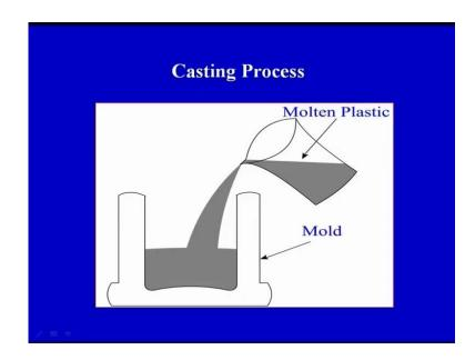
On your screen, you can see a very simple diagram. This is a molten plastic - grey color and it is poured into the mold - this is the mold. The molten plastic is been poured into the mold. The final product that will come out will be according to shape of this mold. So, most simple process, we have a plastic, we are melting it, a molten plastic is being poured into the mold, the final shape of the product would depend upon the shape of the mold.
