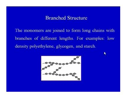
Then we have a branch structure in which the linear structure have branches also. You can see the monomers are joined to form long chain with branch of different lengths, we can see this is a branch, this is a another branch, this is a another branch. So, the length of the branch may be different, so the monomers are joined to form long chains, with branches of different length. So, what are the examples of branched structures? Low density, poly ethylene, glycogen and starch.
