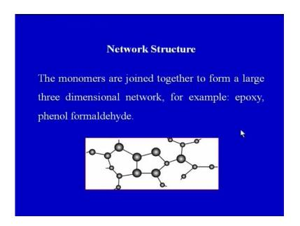
Finally, we have the network structure. The monomers are joined to form a large 3 Dimensional network. For example, epoxy or phenol formaldehyde. So, here also we can see, a epoxy has got a large 3 Dimensional network. And therefore, one important point that has been emphasized today in the lecture itself, that when we combine an epoxy with a hardener and make it cure it into the final product, the final product cures irreversibly.
