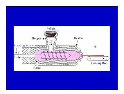
So, basically we can try to understand the basic working principle of the extrusion. This is the screw type of extruder, this is the final part that is coming out. So, depending upon the opening here, we can get the final ceramic part. Depending upon the shape of the opening we will get the shape of the final ceramic part, that part can be further be subjected to other operation, even shaping operations to give it the desired shape, but
