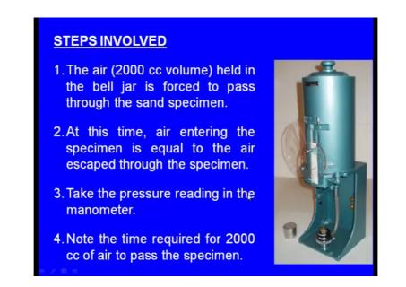
What are the steps involved 200cc volume of air held in the bell jar and it is forced to pass through the sand specimen, at this time air entering the specimen is equal to the air escaped through the specimen, take the pressure reading of the manometer right. Note the time required for the 200 cc of air to escape through the specimen, now permeability can be measured like this.
