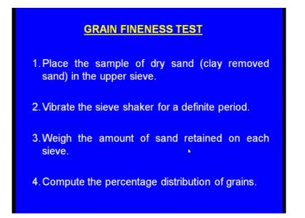
Now this is the way place the sample of dry sand after removing the clay in the upper sieve.
