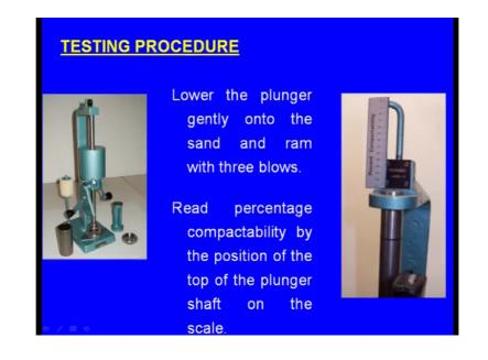
Now, when we place the specimen tube with sand and we can give rams generally lower the plunger and gently on to the sand and ram 3 blows, 3 rams have to be given. Then what happens this is the accessory to measure the what say this compatibility, now this accessory will be fitted here now when we give the 3 rams certainly there will be reduction in the height of the sand .
