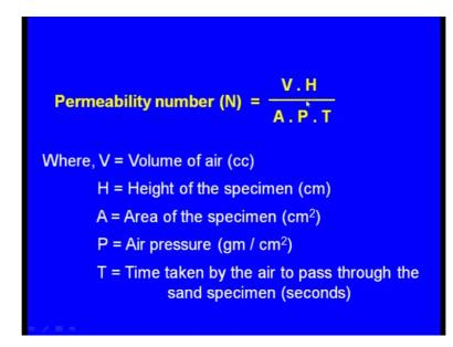
Permeability number is equal to V H divided by A P T, where V is the volume of the air, H is the height of the specimen in centimetres, A is the area of the cross sectional area of
