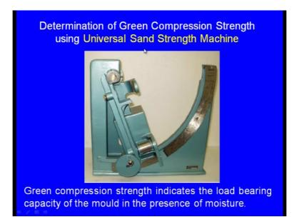
Now, there is a universal sand strength machine is there, you can see this is the universal sand strength what say machine. Now we have to prepare the sand specimen yes this is the tube and in the in to that we have to place the moulding sand and using the rammer and we have to make the rams and the sand will be compacted and here we can see the what say specimen separator.
