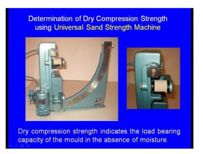
What happens as the machine what say pendulum is going up, what happens previously compression force was falling on the specimen.
