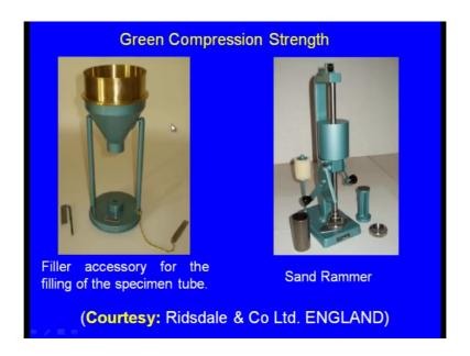
So, let us see how to measure the green compression strength for measuring the green compression strength also we have to prepare the sand specimen, in the same way yes this is the sand what say tube specimen tube and in this we have to place the moulding sand.
