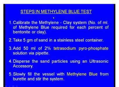
Steps in Methylene blue test, first one what we have to do is we have to calibrate the Methylene with the clay system. So, this Methylene blue solution reacts with the active clay, so as long as the active clay is present right. So, this Methylene blue will be reacting and we cannot see any Methylene blue and it is effects.
