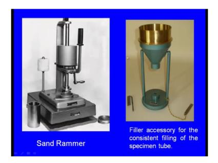
So, this is the specimen tube it is a cylindrical tube and inside this is what say specimen tube we placed the sand, for placing the sand effectively we place the tube here take this tube and put it here. So, this is the filler accessory and through this of funnel we what say drop what say green sand and the grain sand green sand will be dropping inside this specimen tube and now we place this specimen tube here, so this the sand rammer.
