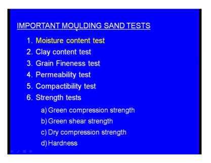
These are the important moulding sand tests, one is the moisture content test another one is the clay content test, next one the grain fineness test, next one the permeability test, next one the compatibility test finally, the strength tests and among the strength test there are 4, one is the green compression strength, green shear strength, dry compression strength and finally the hardness.
