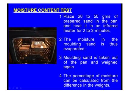
So, this moisture content can be measured using an infrared heater. So, we can see here this is an infrared heater and yes here we can place the sand spaceman.
