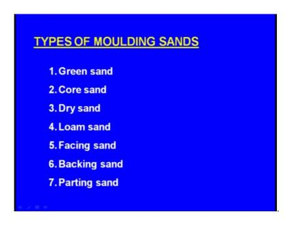
These are the different types of the moulding sands, one is the green sand second one is the core sand, next one the dry sand, next one the loam sand, next one the facing sand, next one the backing sand and finally, the parting sand. Most of the times we hear these a words and some people may not be able to distinguish among these different to sands. Let us see what is the purpose of each and every sand which is mentioned here first let us see the green sand.
