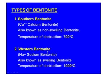
These are the types of the Bentonite; one is the southern bentonite and another one is the western Bentonite. Southern bentonite is also known as calcium bentonite it is also known as non swelling bentonite and it is the temperature of destruction is 700 degrees centigrade. Coming to the western bentonite it is also known as sodium bentonite and it is temperature of destruction is thousand degrees centigrade.
