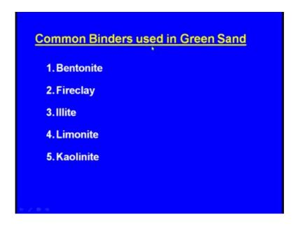
These are the common binders used in the green sand, one is the Bentonite another one is the fireclay next one Illite, next one Limonite, next one Kaolnite. So, these are the common binders used for the green sand mixing now let us see all these binders one by one.
