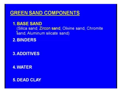
So, we have seen the silica sand what is it is source and what is it is chemical composition and what are it is properties and applications we have seen for the silica sand.
