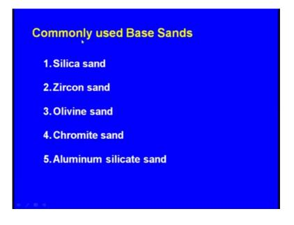
What is this base sand commonly these are the commonly used to beese base sands, one is the silica sand, second one is the zircon sand, third one olivine sand.
