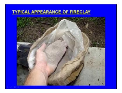
So, this is the typical appearance of the fireclay, next one we will see the illite. Illite is found in natural moulding sands that are formed by the decomposition of micaceous materials due to weathering right. So, it is found right in the natural moulding sands.
