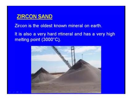
Now, let us see it for the zircon sand. Zircon is the oldest mineral available on the earth are known on the earth. It is also very hard mineral and has a very healthy high melting point that the melting point is 3000 degree centigrade.
