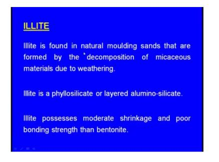
Illite is a phyllosilicate or layered aluminium silicate here also we can see the word phyllo. Phyllo means layers a what say layered on leaf like structures illite possesses moderate shrinkage and poor bonding strength than the bentonite. So, a bentonite is widely use next bentonite this illite is used.
