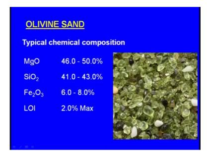
It contains silicon dioxide 41 to 43 percent, it contains iron oxide 6 to 8 percent and it also contains loss on ignition up to 2 percent maximum 2 percent.
