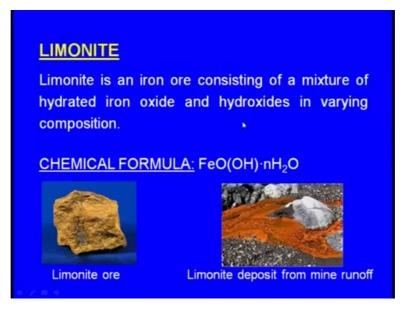
Next let us see the limonite. Limonite is an iron ore consisting of a mixture of hydrated iron oxide and hydroxides in varying composition right. So, the chemical composition is FeO OH and n H 2 O right this n varies right and this is the limonite ore and a limonite deposit from the mine and here we can see this is the limonite deposit. So, this limonite is the another binder used for developing the strength and the cohesiveness of the moulding sand finally, we will see the kaolinite.
