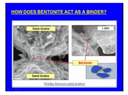
Here we can see this is the bentonite it what say acts as a bridge between the sand grain and sand grain, what say it what say holds both the sand grains together by forming a bridge and same thing we can see here also. So, that is how it makes a bridge between the sand grains and holds them together that is how it improves the cohesiveness of the moulding sand.
