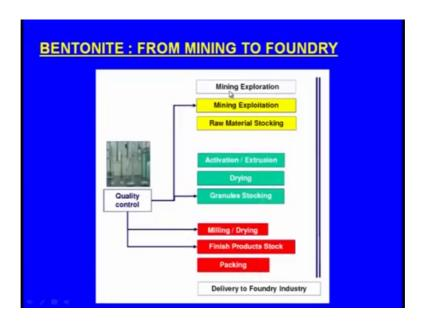
We can see here next one activation next one drying right next one stocking and finally, we can see a milling right.
