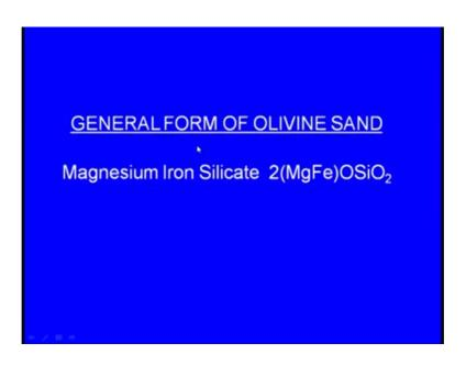
And this is the general form of the olivine sand it is the general form is the magnesium iron silicate 2 Mg Fe O SiO 2. So, this is the chemical composition general chemical composition of the olivine sand.
