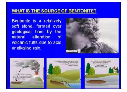
So, bentonite comes from the what say volcanic toughs. So, this volcanic say toughs are on a laid underground for several years and over that we can see acid rains or alkaline rains will be there and because of that we get the Bentonite, and bentonite will be inside the ground and we can take it out side that is the source of the bentonite and this is how we can get the bentonite.
