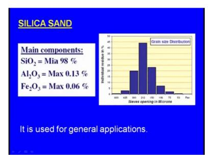
One component is silicon dioxide and it is present up to 98 percent, again it contains aluminium oxide maximum it contains 0.13 percent and also it contains iron oxide up to 0.06 percent and say this is the distribution of the silica sand and it is used for all the general applications.
