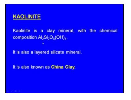
Kaolinite is a clay mineral with the chemical composition alumin Al o 2 SiO2 O 5 and in brackets it is OH4. So, this is the chemical composition of the kaolinite.
