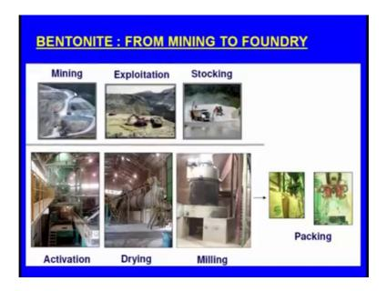
So, next this is the exploitation right with missionary we have to take it that material. Next one and this is this the stocking, next one it is the activation and after that there will be drying and milling finally, it is the packing. So, this is the right a bentonite from mining to the foundry right. So, here we can see first stage is the mining exploiration exploration, next one mining exploitation, next one raw um me material stocking.
