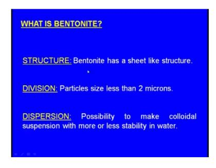
Next one it is a structure bentonite has a sheet like structure just now we have seen right and it is the division particle size is less than two microns. Dispersion possibility to make colloidal suspension with more or less stability in water. Now what is the source of Bentonite? Bentonite is a relatively soft stone formed over geological time by the natural alteration of volcanic tough due to acid or alkal alkaline rain.
