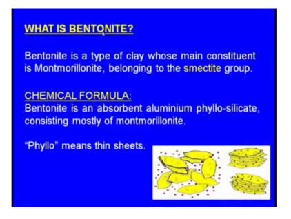
First of all what is this Bentonite? Bentonite is a type of clay whose main constituent is right montmorillonite belonging to the smectite group, and what is it is chemical formula? Bentonite is an absorbent aluminium phyllosilicate consisting mostly of montmorillonite here we can see word Phyllo. Phyllo means thin sheets means it is available in the form of thin lamellar sheets that is the physical structure of the bentonite.
