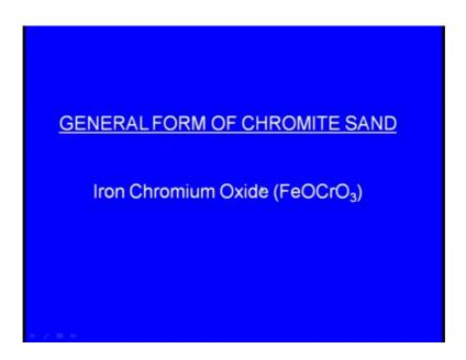
So, these are the different what say elements or the different components present in the chromite sand. This is the general form of the chromite sand it appears as the iron chromium oxide FeO C r O3. So, this is the general form of the chromite sand. We have seen silica sand zircon sand olivine sand chromite sand now let us see the aluminium silicate sand aluminium silicate right.
