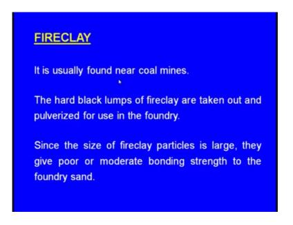
It is usually found near the coal mines right the hard black lumps of fireclay are taken out and pulverized for use in the foundry. Since the size of the fireclay particles is very large they give pour or moderate bonding strength to the foundry sand right. So, it is used all right usually found near the coal mines. (Refer Slide Time: 41:15).
