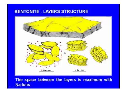
And here we can see it is present in the form of the sheet like structure layered structure and we can see this is the sodium ion and here we can see calcium ion. The space between this layers is maximum with the sodium ions how does bentonite act as a binder that is the next question, and here we can see this is a sand grain this is a sand grain and this is a sand grain and.
