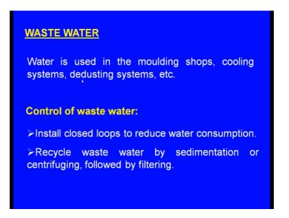
Water is used in the moulding shops, cooling systems, dedusting systems and so on. In the molding shops we use the water and in the cooling systems we use the water, dedusting system we use the water, at every stage water is polluted. Now control of wastewater install closed loops to reduce water consumption. Next one recycle waste water by sedimentation or centrifuging, followed by filtering.
