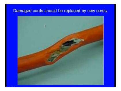
A damaged cord you see and here we can there is a leakage is there you see here we can see the core wire. So, these kind of cords could cause what say electrical accidents and injuries.
