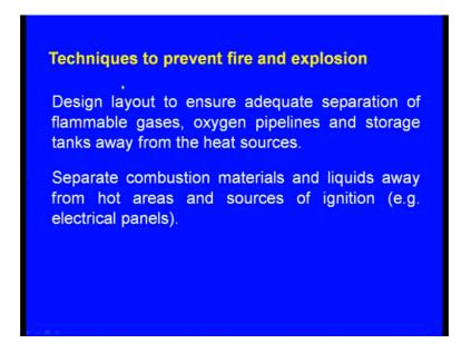
Techniques to prevent the fire and explosion: Design layout to ensure adequate separation of flammable gases, oxygen pipe lines and storage tanks away from the heat sources, next one separate combustion materials and liquids away from hot areas and sources of ignition example electrical panels. So, these are the few techniques to prevent fire and explosion. (Refer Slide Time: 40:56)
