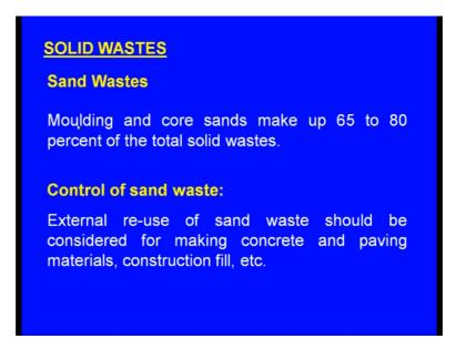
Moulding and core sands make up to 65 to 80 percent of the total solid wastes. You see the molding sand and the core sand are contributing 65 to 80 percent of the total solid wastes.
