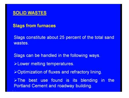
Now, under this solid waste let us see the slags from the furnaces: First one is the what; say foundry sands so they contribute to the maximum percent of the solid wastes from the foundry. The next solid waste is the slags from the furnaces; slags constitute about 25 percent of the total sand wastes.
