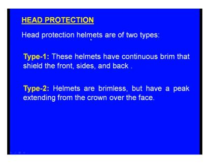
Head protection helmets are of two types: you see type 1 and type 2. In the type one these helmets have continuous brim that shield the front sides and back. In the type two helmets are brimless but have a peak extending from the crown over the face.
