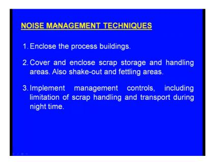
Noise management techniques: First one is enclose the process buildings, cover and enclose scrap storage and handling areas. Also shake out and fettling areas. Implement management controls, including limitation of scrap handling and transport during night time.
