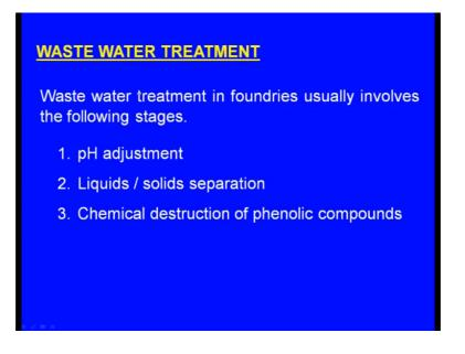
Now let us see the waste water treatment. This is very important wastewater treatment in foundries usually involves the following stages one is the pH adjustment liquids, solids separation and finally chemical destruction of phenolic compounds.
