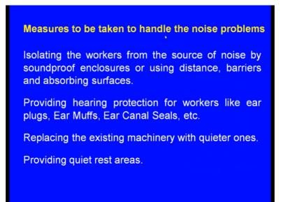
Measures to be taken to handle noise problems: Isolating the workers from the sources of noise by sound proof enclosures or using distance, barriers and absorbing surfaces. Providing hearing protection for workers like ear plugs, ear muffs, ear canal seals and so on. Replacing the existing machinery with quieter ones providing quiet rest areas so these are the measures to be taken to handle the noise problems.
