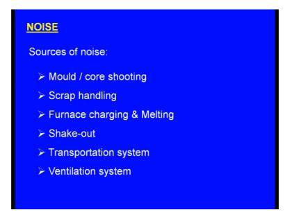
Sources of noise: What are the sources of noise? Mould core shooting, scrap handling, furnace charging and melting, shake-out, transportation system, ventilation system.
