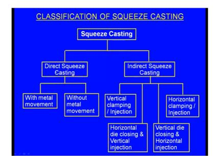
And the squeeze casting we have seen, there are 2 types: one is the Direct what say Squeeze Casting and the other one is the Indirect Squeeze Casting. Again, direct squeeze casting is classified as with metal movement and without metal movement. Indirect squeeze casting is classified as Vertical clamping, Vertical Injection, Horizontal closing and Vertical injection, Vertical die closing and Horizontal injection and finally, horizontal clamping and Injection.
