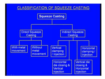
So we have seen, the difference between the direct squeeze casting process and the indirect squeeze casting process. Now let us concentrate on the direct squeeze casting process. So under the direct squeeze casting process, we have 2 types one is the with metal movement and the other one is the without metal movement. Let us see, what are these?
