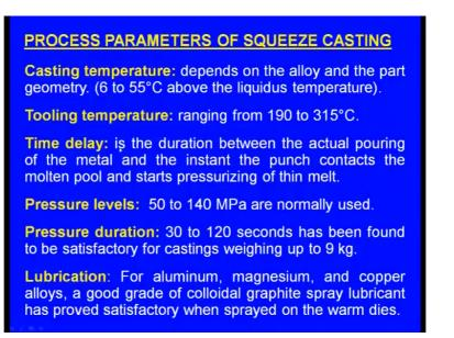
Now what are the process parameters of squeeze casting process? One is the Casting temperature. Now, this casting temperature depends on the alloy and the part geometry and this casting temperature should be 6 degrees to 55 degrees centigrade above the liquidus temperature.
