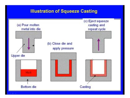
So, this is the die metallic die and here this is the upper die and here we can see the molten metal is poured into the die. Then, the upper die comes down and presses. Yes, it has pressed here. We can see here and you remember this pressure will be applied till the molten metal is completely solidified. Yes, after sometime the molten metal will be completely solidified. Then, the upper die will be withdrawn and it will be going up. Now this is the solidified casting.
