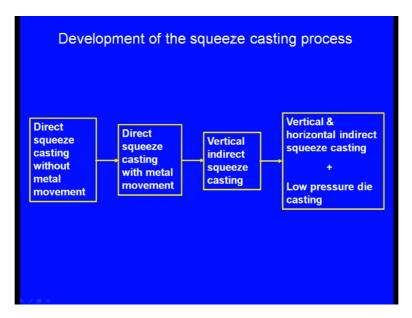
What are the steps involved? We have seen that what say squeeze casting is there are different types of squeeze casting process; one is the direct squeeze casting without metal movement or direct squeeze casting with metal movement or so on. What to use, when? We can see here, this is the block diagram for the whatsay use of the different process.
