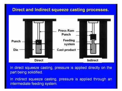
So here, we can see this is the direct squeeze casting and this is the indirect squeeze casting and here we can see, this is the die, this is the die and here also this is the die. Now this is the punch here, this is the punch and here also, this is the punch. Now the molten metal, this is the die and the molten metal is poured here and the punch is coming down and it is applying pressure on the molten metal. And here we can see, this is the molten metal.
