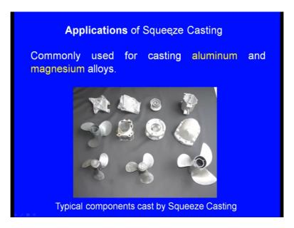
Now these are the typical applications of the squeeze casting. Now it is commonly used for casting aluminum and magnesium alloys. Remember, squeeze casting is used for aluminum and magnesium alloys and these are the typical components produced by squeeze casting process, you can see here. So this is a whatsay fan blade. So, all these are made by squeeze casting process. (Refer Slide Time: 33:33)
