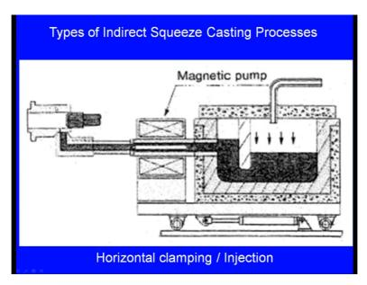
Finally, Horizontal clamping and Horizontal injection and here we can see these, these are the dies, these are the dies and they are closed what say clamped horizontally and this is the whatsay punch.
