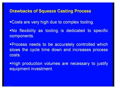
Now, these are the drawbacks of squeeze casting process. Costs are very high due to complex tooling. No flexibility as tooling is dedicated to specific components. So that tooling means these dies are meant for making particular components. If we want to
