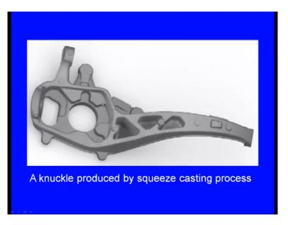
A knuckle produced by squeeze casting process, you can see here. It has got very fine details and this is produced by squeeze casting process.
