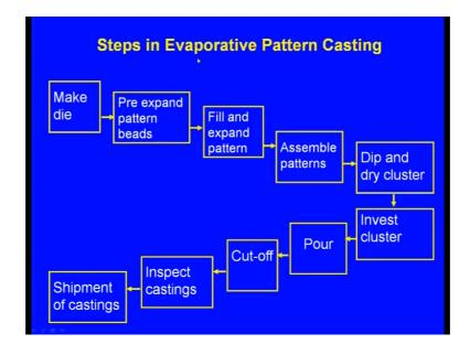
Now, these are the steps involved in the evaporative pattern casting process. First step is Make the die, second step pattern expands pre expanded what say pattern Pre expand pattern beats. First step is Making the die, second step is Pre expand pattern beads, next one Fill and expand patterns, third step Assemble patterns, fourth step Dip and dry cluster. We have to make the ceramic slurry. So in that ceramic slurry, the assembly, are the patterns will be dipped and it will be clustered.
