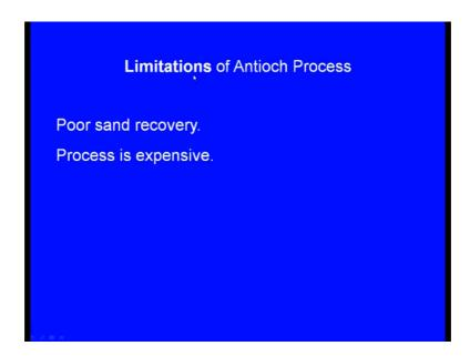
Improved mechanical properties but what are the limitations of this Antioch process? Poor sand recovery. So that is the drawback of this process and process is expensive. Again we have to mix the fine silica sand. It is not in the case of the sand, sand casting process the entire sand can be recovered, only little sand is what is burnt. So there is a sand loss, but most of the times most of the sand is reused it is recovered, but here the
