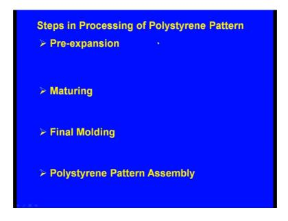
Now the steps in processing of the polystyrene pattern, so these are the steps for processing the polystyrene pattern. One is, the first step is the Pre-expansion, second step is Maturing, third step is Final Molding, fourth step is Polystyrene Pattern Assembly. Now let us see what are these.
