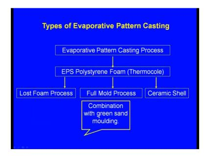
In the case of the full mould process, the pattern is packed with the green sand molding process. So that way, this is a combination with green sand molding. And let us see what is this ceramic shell?
