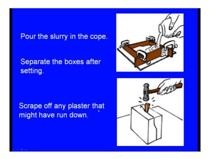
Next one pour the slurry in the cope. In the similar way, we have to make the cope also. Now again 4 boxes will be kept, now pour the slurry in the cope. Separate the boxes after the setting. Now you see this is the mould. Now scrape off any plaster that might have run down, if any plaster is unnecessarily occupying anywhere that must be scrapped off or that must be broken and eliminated.
