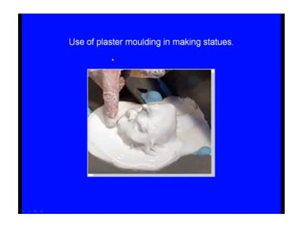
And here we can see, use of plaster moulding in making statues for making art castings. So initially, when one has to make the plaster mould into that plaster mould one has to pour the molten metal then, we get the statues like this.
