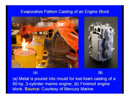
Now here, we see a drain what say real application for making engine block. So this is the engine block. So here we can see, metal is poured into mould for a last firm casting of a 60-hp 3-cylinder marine engine. Here we can see one a one mould box is there, only one molding box and this is the pouring cup and the molten metal is being poured and as
