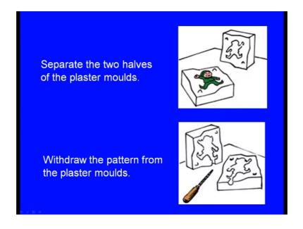
Separate these two halves of the plaster molds. So these must be separated. Now pattern is still inside, you can see. Now withdraw the pattern from the plaster moulds, this pattern is withdrawn, using a screwdriver or somewhat say appropriate tool.
