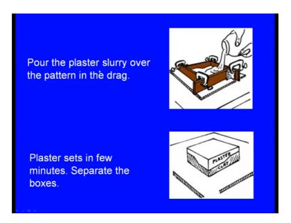
Now pour the plaster slurry over the pattern in the drag. So inside there is already a pattern, now around the pattern, we have placed with the molding box. Now pour the plaster, plaster slurry over the pattern in the drag molding box. Now this plaster will be setting in few minutes, after that the on the 4 sides, there are 4 what say boxes are there right. So these must be separated.
