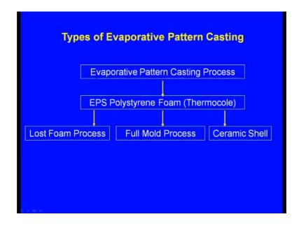
Now, these are the types of evaporative pattern casting. So in this evaporative pattern casting process EPS Polystyrene Form or the Thermocole is used as the pattern material. Now broadly this can be classified into 3 types. One is the Last Foam Process means this is the one which is widely used nowadays. The second one is the Full Mould Process which was used in the beginning, but now also it is used and finally, the Ceramic Shell process.
