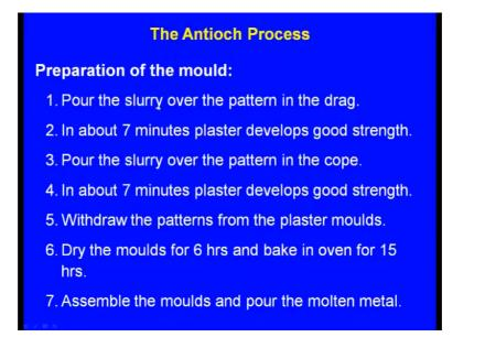
Now preparation of the mould, Pour the slurry after we prepare the slurry, pour the slurry over the pattern in the drag. In about 7 minutes plaster develops and gains a good strength. Pour the slurry over the pattern in the cope also in the same way. In about 7 minutes plaster develops and gets a good strength. Next one withdraw the patterns from the plaster moulds as usual. Now dry the moulds for 6 hours and bake in oven for 15 hours. Assemble the moulds and pour the molten metal.
