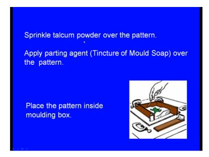
Second step sprinkle talcum powder over the pattern. So this is the pattern, over the pattern sprinkle talcum powder. So that, the slurry, may not be sticking in to the pattern. Next one apply parting agent Tincture of Mould Soap over the pattern. So this also will enable us to prevent the sticking of the slurry with the pattern. Now place the pattern inside the molding box. So this is the molding box, inside this molding box, place the pattern.
