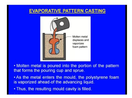
Molten metal is poured into the portion of the pattern that forms the pouring cup and sprue and here we can see this whole thing is the pattern and this is the pouring cup. So this process is somewhat different from the other process. In one sense that in all the previous process so before pouring the molten metal, we remove the, withdraw the pattern from the mould. But here, the most specialized special feature is that we will not remove the pattern from the mold.
