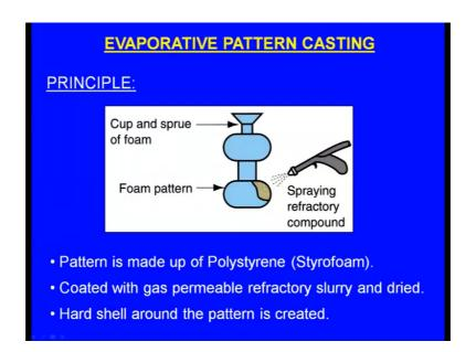
So here, the pattern is made up of Polystyrene or Styrofoam. So this is the polystyrene pattern or the Styrofoam pattern and here we can see the pouring cup is there and this is
