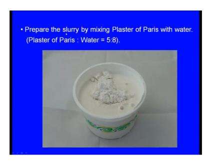
Now prepare the slurry by mixing Plaster of Paris with water. So that is the first step in the conventional plaster molding process. Now Plaster of Paris and water proportions are 5:8 means Plaster of Paris should be 5 parts and water should be 8 parts. So prepare that slurry by mixing these two ingredients.
