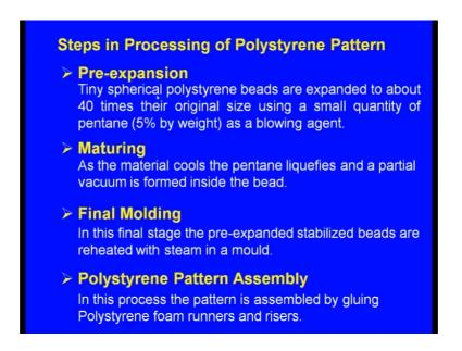
In the case of the Pre-expansion, Tiny spherical polystyrene beads are expanded to about 40 times their original size using a small quantity of pentane and its proportion is 5 percent by weight as a growing agent. Now the second step is the Maturing. What is this?
