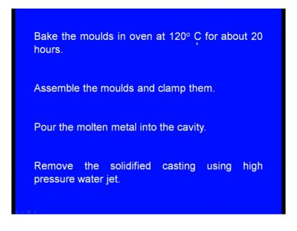
Bake the moulds in an oven at 120 degree centigrade for about 20 hours. So this must be baked. So that the moisture will be evaporating and also the plaster moulds will be hardened. Assemble the moulds and clamp them. After that these 2 moulds must be assembled and they must be clamped together. Pour the molten metal into the cavity after pouring after so right, after solidification; remove the solidified casting using high pressure water jet.
