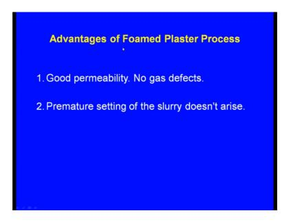
Good permeability, no gas defects. Because we have what say filled half of the slurry with the air bubbles because of that the permeability is enhanced significantly. Next one premature setting of the slurry does not arise; these are the disadvantages of the foamed plaster process.
