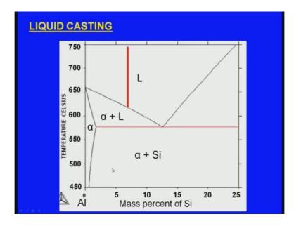
And here in this what say this is the phase diagram of aluminum and silicon and here we can see this is the liquidus temperature and this is the solidus temperature and here we can see this is the mixture of liquid and solid. Now, if you do the liquid casting the casting is carried out above the liquidus temperature. So, this is the liquidus temperature.
