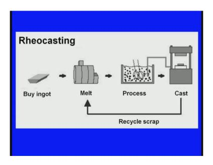
Now, what are the advantages of rheocasting process? No need to buy the pre cast billet us as in the case of the thixocasting. So, because we are buying the precast billet us in the thixocasting process the process becomes expensive. So, such things will not arise here in the case of the rheocasting. Scrap can be reused immediately, immediately if there is any scarp again it can be what say kept inside the furnace and we can get the required slurry.
