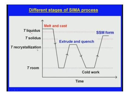
Now, here we can see this process diagrammatically. Now, this is the liquidus temperature and this is the solidus temperature and this is the re crystallization temperature and this is the room temperature. Now, you see here initially it is in the molten state. Now, then it what is happening it is what say deformation is taking place right.
