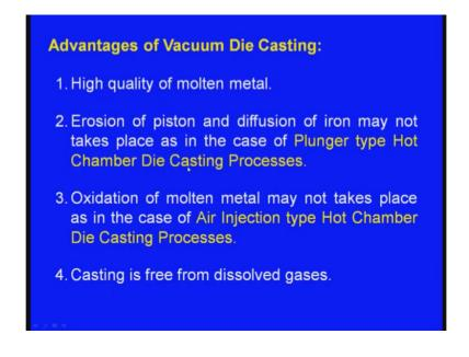
Next one erosion of piston and diffusion of iron may not takes place as in the case of the plunger type hot chamber die casting process. Now, in the case of the plunger type hot chamber die casting process what is happening we apply the pressure on the what say plunger that plunger goes inside the what say that is cylindrical barrel as it comes down the molten metal will be injected inside the two dies.
