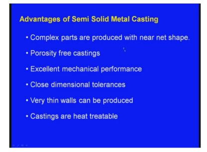
Now, let us see the advantages of semi solid metal casting process complex parts are produced with near net shape very complex parts can be produced. Near net shape means almost no machining or negligible machining is required.
