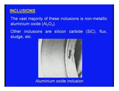
And here can see aluminium oxide inclusion next one gas porosity under the internal defects gas porosity is due to trapped gases. Now, what are the sources of these gases trapped air in the furnace air in the cold chamber or gases from excessive lubricants, we use lubricants. So, that time also from the lubricants gases will be arised.
