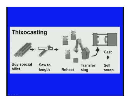
Now, this is what we can say diagrammatically. So, these are the special billet us pre cast billet us. So, these are available in the market which are manufactured with under certain what say special conditions it has got the non dendritic micro structure. Now, we will be cutting this saw to the required length and also to the required quantity we will cut them.
