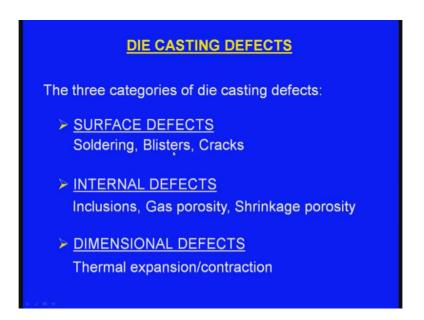
One category first category is the surface defects, second category internal defects, third category dimensional defects. Under the surface defects we have soldering blisters and cracks, under the internal defects we have inclusions gas porosity and shrinkage porosity, under the dimensional defects there will be thermal expansion or contraction.
