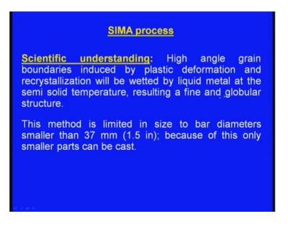
This method is limited in size to bar diameters smaller than 37 millimeters because of this only smaller parts can be cast, so that is the limitation of this process only smaller components can be cast.
