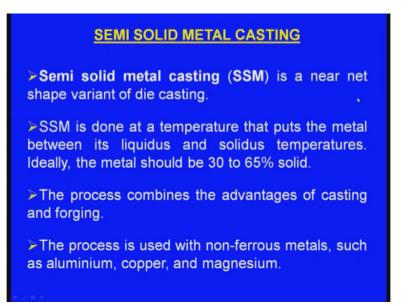
Now, what are the features of semi solid metal casting? Semisolid metal casting is a near net shape variant of the die casting process. Semisolid metal casting is done at a temperature that puts the metal between its liquidus and solidus temperatures, ideally the metal should be 30 to 65 percent solid means it is not totally solid it is not totally liquid.
