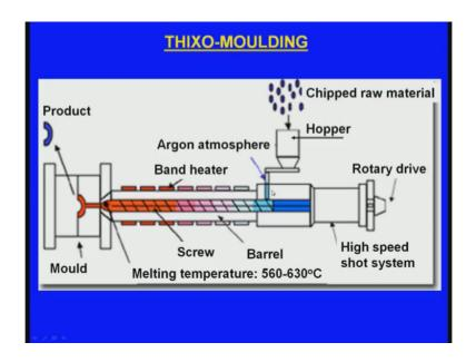
And what is this machine? It has a barrel you see this is a barrel outside barrel. Now, inside there is a screw it rotates and this is connected to a motor you see here, here it is connected to a motor and here there is a feeding hopper. So, there is a hopper will be there to feed the magnesium alloy chips here we feed the magnesium alloy chips.
