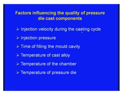
Now, let us see the factors influencing the quality of pressure die cast components one is the injection velocity during the casting cycle, next one injection pressure, next one time of filling the mould cavity, next one temperature of cast alloy, next one temperature of the chamber and finally, temperature of pressure die.
