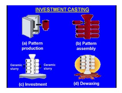
Now, this is the a what say simple principle of the investment casting. Investment casting process means the pattern is made up of wax in the olden days the ancient man when he wanted to manufacture these spear heads or the rudimentary tools, he initially he made a wax pattern around the wax pattern he has compacted the sticking sand later he has heated that to system and the wax has a drained out inside there was a cavity, into that cavity the molten metal was poured.
