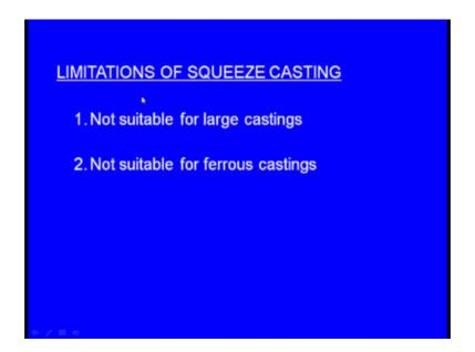
These are the limitations of the squeeze casting process, not suitable for the large castings because the moulds are made up of the a special dies metallic dies. So, very large castings cannot be made, not suitable for the ferrous castings because the metallic dies are made up of ferrous alloys. So, it can be used one way for the non ferrous castings.
