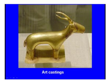
Now, you see its complex features, if you make this by any other casting process it will have a rough surface. Once there is a rough surface we need to machine it, now it is not possible to machine this under a machine, but when you make this using the investment casting process the way already we get a very smooth surface. So, there is no need to machine it. So, investment casting is also used in the art castings, next one let us see the continuous casting process.
