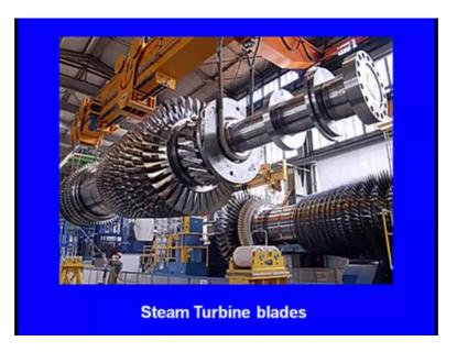
And here we can see these a steam turbine blade which is used in a thermal power plant, you can see this is the turbine blade it is a very huge turbine blade and you can see these are all the blades these are all the blades and all these blades are manufactured by investment casting.
