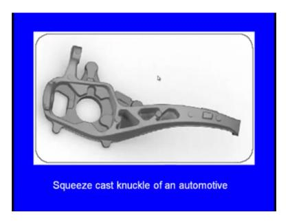
And here we can see the typical what say components produced by the squeeze casting process and this is this squeeze casting knuckle of an automotive.
