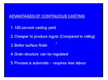
We get the 100 percent casting yield, first of all what is meant by casting yield. Suppose in by if you make a casting by green sand moulding suppose if the weight of the casting is 100 kgs, we pour more than 100 kgs of the molten metal because the molten metal occupies into the sprue and also into the riser. So, if we want to make a casting of 100 kgs about to 125 kgs of molten metal we pour into the cavity.
