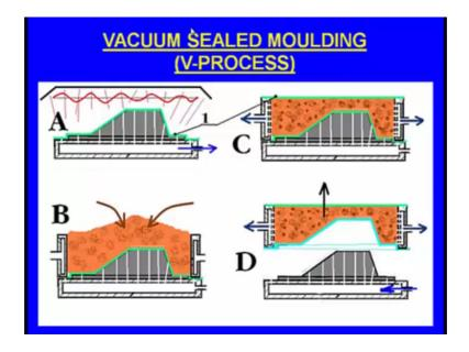
Here we use vacuum to bind the or to hold the moulding sand whereas, in the case of the green sand moulding we will used to mix some binders and place moisture. So, that some binding action will be developed between the moulding sand and such a sand we what say place inside the moulding box and when we compact yes we get a moulding cavity and here we want use the what say clay or any binder even the moisture we want use, we use a fine and dry sand and here we use vacuum to hold the sand.
