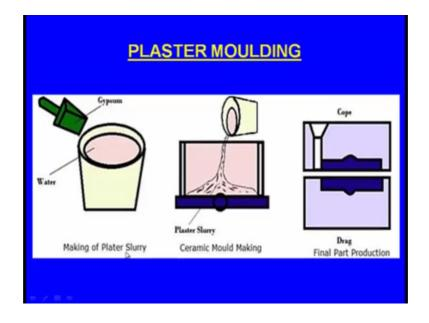
So, initially we have to prepare the plaster of Paris, these also known as the gypsum commercially. So, this will be mixed with water and we prepare a what say slurry plastic of Paris or the gypsum slurry we prepare in a container and we yes we place the pattern here. So, this is the pattern and we pour the what say plaster of slurry here around about
