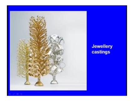
So, this is that central tree or this sprue and through this they are pouring the molten metal and. So, these are all the individual castings of course, finally, they will separate all these individual castings. So, these jewellery items are manufactured by investment casting.
