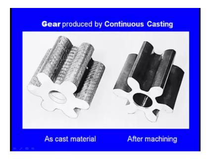
gear blanks this is a gear blank, this was manufactured by continuous casting means inside there is a mould in the cross section of the mould was similar to the gear blank profile and this is the as cast material afterwards it was machined and after machining we got a gear like this. So, gears are also manufactured by continuous casting.
