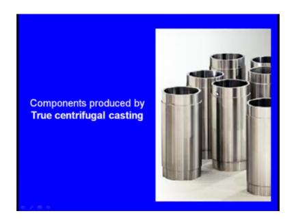
We can see. So, these are all the components produced by the true centrifugal casting process. Next one let us see the plaster moulding process in the plaster moulding process we use the plaster of Paris.
