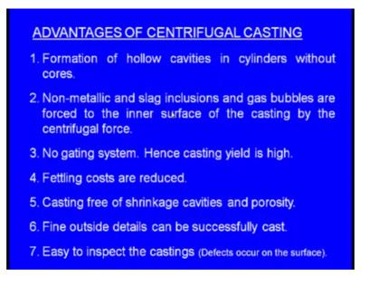
Formation of hollow cavities in the cylinders without cores, if we have to make what say internal cavities in a casting we have to use cores again this cores what are these cores we will be studying in the next lecture. A non metallic and slag inclusions and gas bubbles are forced to the inner surface.
