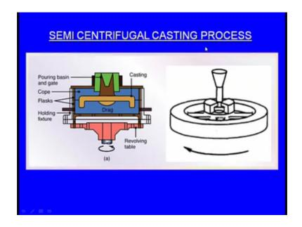
In the semi centrifugal casting process are the system rotates on a vertical axis whereas, in the case of the true centrifugal casting process the mould was rotating on a horizontal axis and here the mould rotates around a vertical axis right.
