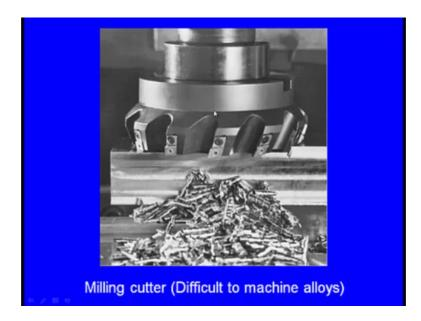
This milling cutter is made up of difficult to machine alloy; most of the times it contains large amount of tungsten and it is very difficult to machine this kind of steel, now this milling cutter is manufactured by investment casting.
