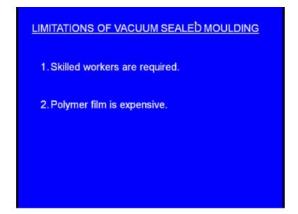
Next let us see the limitations of the vacuum sealed moulding in this process the skilled workers are required, because the vacuum has to be applied in the right time and also it should be applied for the right duration. So, this requires skill, next one the polymer film is expensive and for each casting we have to use new polymer film, once we use polymer film for one casting. So, that is that cannot be used for the next casting. So, that way the process becomes expensive.
