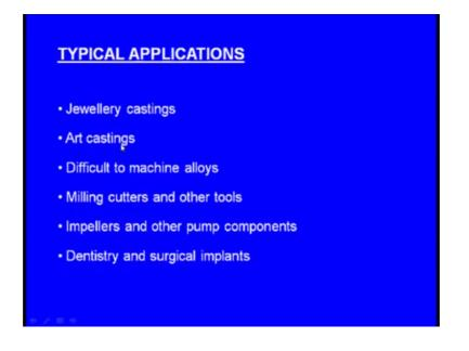
Can be made difficult to machine alloys can be made by investment casting process milling cutters and other tools impellers and other pump components and finally, it is used in the dentistry and surgical implants the artificial teeth are manufactured by the investment casting. (Refer Slide Time: 12:25)
