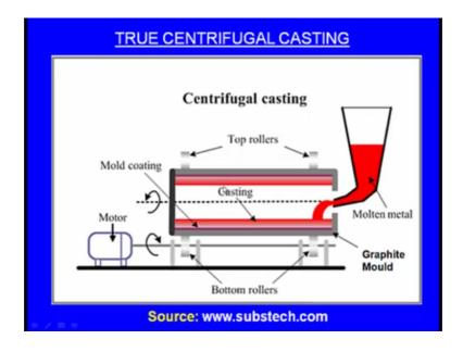
So, this is the centrifugal or true centrifugal casting what is it the principle? There will be a graphite cylindrical mould will be there. So, this is the cylindrical graphite mould the one which is looking in the gray color.
