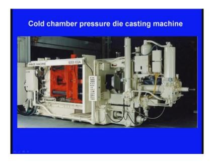
Now, let us see the advantages of cold chamber die casting process. Simple construction, thus cost of the equipment is not very high. What is there? Two metallic moulds are there and yes, there will be ejector pins will be there and a cylinder chamber is there and a piston or a ram and we just pour the molten metal and push it.
