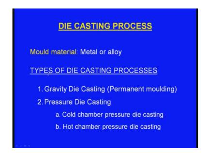
Now, here the mould material is metal or alive. Now, we have seen that in the case of the die casting process a metallic mould will be used and the same metallic mould will be used to make thousands and thousands of castings.
