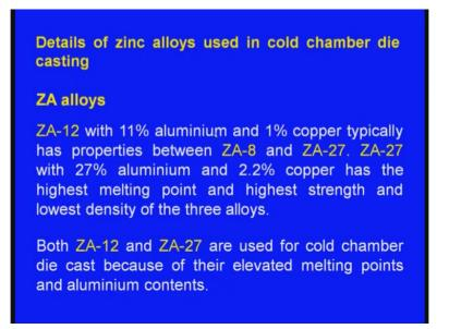
Next one, we will see details of zinc alloys used in hot chamber die casting. ZA alloys ZA-12 with 11 percent aluminium and 1 percent copper typically has properties between ZA-8 and ZA-27 with 27 percent aluminium and 2.2 percent copper has the highest melting point and highest strength, and lowest density of these three alloys. Next one, both ZA-12 and ZA-27 are used for cold chamber die cast because of their elevated melting points and aluminium contents.
