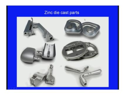
So, these are the zinc die cast parts, you can see excellent surface finish is there. So, these cast parts are made by hot chamber pressure die casting process.
