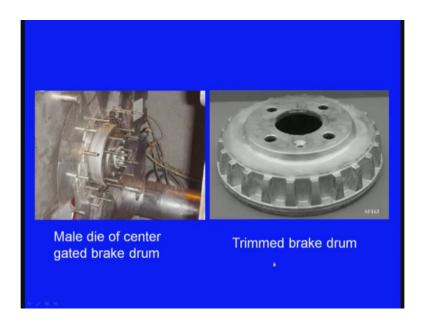
Next one, we can see here, this is the trimmed brake drum. So, this is made by pressure die casting process this is the male die of center gated brake drum, this is the male die. Now, we can see here more examples. So, all this components are made by pressure die casting process.
