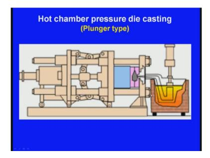
Ha here we can see the animation. So, this is the what say; what say this is the furnace and here we can see the molten metal is going inside, and here we can see the gooseneck plunger is coming down, and these two are the dies the molten metal will be injected inside, immediately there will be a cooling system, to cool the what say casting, and it will be ejected, and the casting will be taken out.
