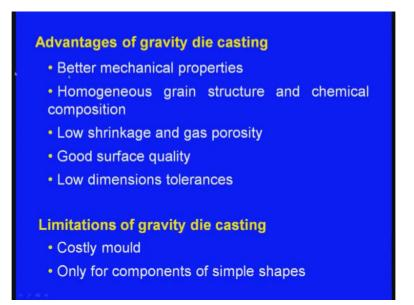
Now, let us see the advantages of gravity die casting, better mechanical properties. Why? the molten metal is being poured into the mecha what say, metallic moulds then what will happen the cooling rate will be faster. Once the cooling rate is faster, we get the mechanical properties. Now so, better mechanical properties are obtained in the gravity die casting.
