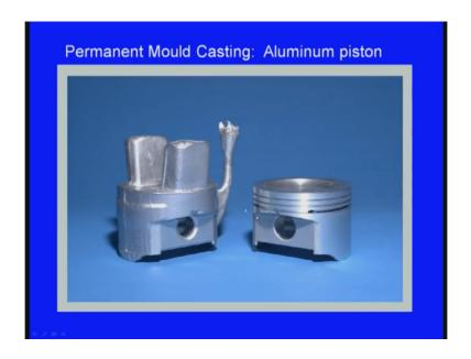
Now, this is the ejected casting permanent mould right, here we can see you can see aluminium pistons. So, these are made by what say permanent moulding.
