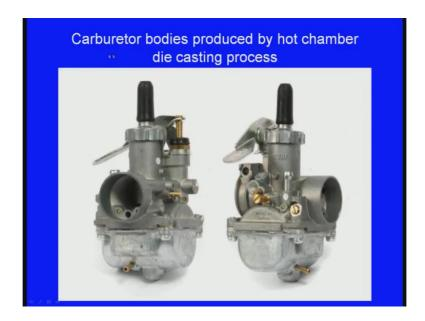
And here, we can see important applications, carburetor bodies produced by hot chamber die casting process. So, these are the carburetor bodies used in the automotives. This is a another component, thin component produced by hot chamber die casting process. So, again this is a, what say cast product of hot chamber die casting process.
