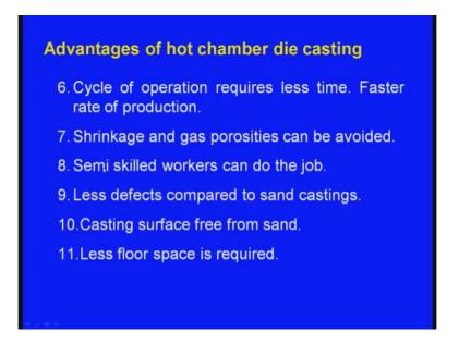
Less defects compared to the sand casting, casting surface is free from sand particles. So, no need to wash, right less floor space is require in the case of the sand casting process, there will be a pattern shop will be there for making the pattern, there will be a moulding shop for making the, what say sand, and there will moulding shop, there will be melting shop, there will be quilting shop, there will be, what say machining shop likewise. So,
