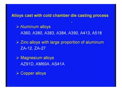
Now, let us see the alloys cast with cold chamber die casting process, A360, A380, A383, A384, A390, A413 and A518. So, these are the alloys which are cast using the cold chamber die casting process. Next one, what are the alloys in among the zinc alloys? What are those alloys? Let us see among the zinc ZA-12, ZA-27 are the zinc alloys which are cast using the cold chamber die casting process.
