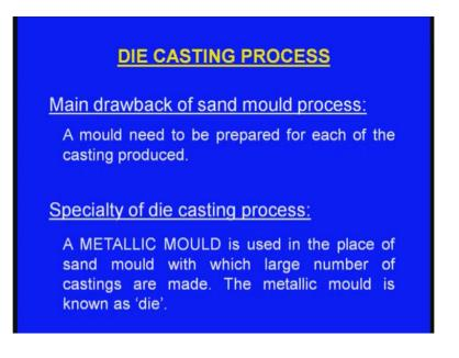
Now, what is this die casting? Why we should go for die casting? Let us see, first of all what is the drawback of sand moulding process? Why we should go, what say live sand moulding, and why we should switch over to die casting.
