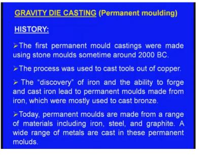
This process was used to cast tools out of copper, those days. Now the discovery of iron and the ability to forge the cast iron lead to permanent moulds made from iron which were mostly used for to cast branch. Now later, men has what say learnt how to melt what say extract iron, how to melt iron, and how to forge iron components, with that they even made permanent moulds permanent metallic moulds made up of iron. So, these were used to cast branch.
