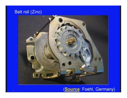
So, this a belt roll it is a zinc, what say casting it is made up of what say pressure die casting process.
