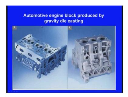
And we can see here automotive engine blocks produced by gravity die casting. So, these are the engine blocks which has used; which are used in the automotives. So, these engine blocks are made by permanent moulding process.
