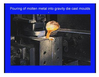
And here we can see pouring of molten metal into the gravity cast moulds, it is being poured. So, this is one die and this is one die.
