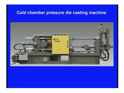
Now, here we can see a cold chamber pressure die casting machine. Another cold chamber pressure die casting machine we can see here, and these are the dies we can see here.
