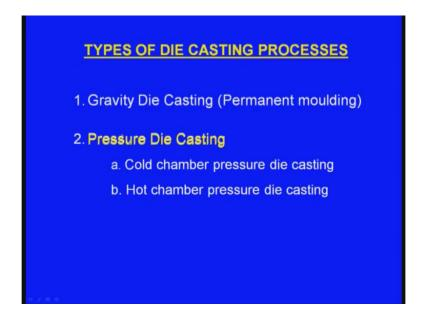
Next one, we have completed the gravity die casting. Next one, we will see the pressure die casting. Again, the pressure casting is sub classified as cold chamber pressure die casting, second one is the hot chamber pressure die casting.
