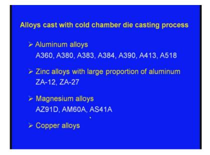
Now, ca alloys cast with cold chamber die casting process. In detail we have seen aluminium alloys A360, A380, A383, A384, A390, A413, A518 coming to the zinc alloys ZA-12, ZA-27 coming to the magnesium alloys AZ91D, AM60A, AS41A and some copper alloys.
