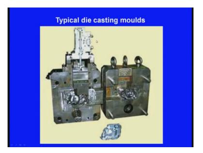
So, this is the world's largest hot chamber die casting machine. These are the typical die casting mould. So, these are the dies, dies means metals moulds which are used in the dia what say hot chamber die casting process.
