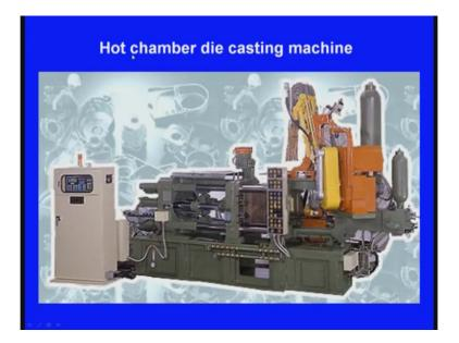
So, this is the, what say animation of the hot chamber pressure die casting process. And here we can see another hot chamber die casting machine and here we can see 8 ton hot chamber die casting machine, this is the largest hot chamber machine in the world, and it costs about 1.25 million dollars. You can see the height its height its height is doubled than the height of an average men, you can see here maybe it must be the height must be the 12 feet and this is the length.
