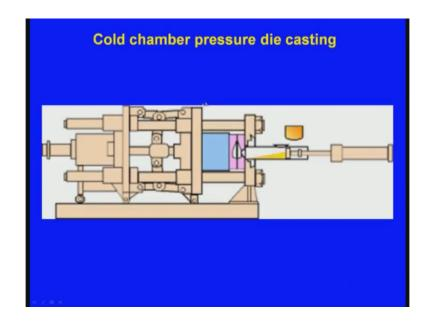
Yes, here we can see, yes this is the casting. Again it will be poured, again it exerts pressure between into the die and casting solidifies and the casting will be taken out.
