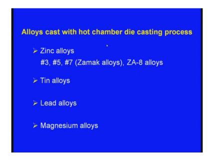
Now, alloys cast with hot chamber die casting process. Zinc alloys can be cast, tin alloys can be cast, lead alloys can be cast, and finally magnesium alloys also can be cast using hot chamber die casting process, and what are those among the zinc alloys, 3 5 7. So, these are the zamak zinc alloys. So, these can be cast using hot chamber die casting process and also ZA-8 alloy can be cast using the hot chamber die casting process.
