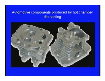
Next one, automotive components produced by hot chamber die casting process. Here we can see these are the automotive components these are produced by hot chamber die casting process. Next one, this is a another component produced by hot chamber die casting process.
