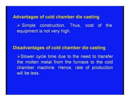
So, it is a simple construction. Then what are the disadvantages of cold chamber die casting process? Slower cycle time due to the need to transfer the molten metal from the furnace to the cold chamber machine. What is this? Sometime back, I told you in the case
