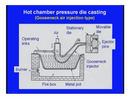
So, you can see here the, here is the molten metal and initially the metallic blocks will be kept inside this furnace in this what say, metal pot. Then here, there is a fire box using this fire box there will be coke or oil it will be burnt and because of that the molten blocks will be melted and there will be molten metal will be there. So, here we can see that the what say, furnace is an integral part of the machine.
