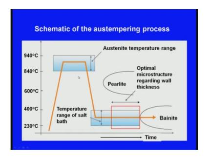
Now, we will see the diagram. So, this is the schematic diagram of the austempering process.
