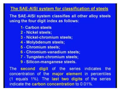
Now, the SAE the society for automotive engineers and AISI, american iron and steel institute system for classification of steels the SAE, AISI system classifies all other alloy steels using 4-digit index as follows, right? One means one series, these are the carbon steels. 2 series means, nickel steels means nickel is the principle alloying element other elements also will be present 3 series means nickel chromium steels. 4 series means, molybdenum steels.
