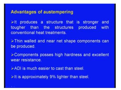
Now, what are the advantages of austempering or the austempered ductile iron? It produces a structure that is stronger and tougher than the structures produced with conventional heat treatments. Thin walled net shape components can be produced why?
