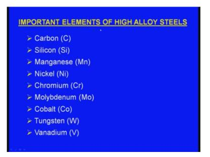
Now, important elements of high alloy steels. What are the elements or the principle alloying elements present in the high alloy steels? One is the carbon may not be the what say primary element or the principle alloying element, but these are present carbon is
