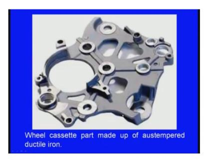
Now, this is a typical example of ductile, what say austempered ductile irons application a wheel what say cassette part made up of austempered ductile iron.
