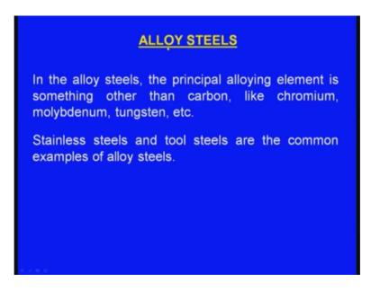
Next one let us see the alloy steels. Now what are the characteristics of alloy steels? In the alloy steels the principle alloying element is something other than carbon. Like, chromium, molybdenum, tungsten etcetera. It does not mean that carbon is not present. Carbon will be present, but or the rather than the carbon the influence of some other element will be dominating.
