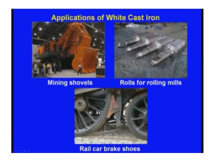
So, these are the mining shovels. So, these are made up of white cast iron. These are the rolls for rolling mills. Again, these are made up of white cast iron. Now this is the rail car brake shoes. Here we can see this is the rail car brake shoe. Now if it is the ordinary cast iron what will happen? It will be what say undergoing the wear, but white cast iron has got the excellent wear resistance. Because of that nothing will happen, even when we apply the brake.
