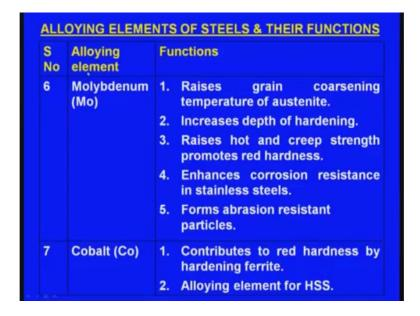
Next one it increases hardenability. It increases strength at high temperatures. Now with higher carbon.
