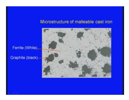
Here the matrix is the ferrite we can see here this is the ferritic may what say matrix, and this is the graphite packet or the carbon packet, this one.
