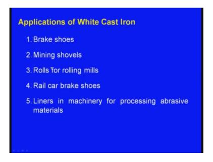
Now, these are the common applications. In fact, important applications of white cast iron. Brake shoes, mining shovels, rolls for rolling mills, rail car brake shoes, liners in machineries for processing abrasive materials. We will see few pictures.
