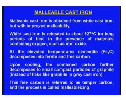
Now, finally, we will see the malleable cast iron. Malleable cast iron is obtained from white cast iron, but with improved malleability. It is obtained from white cast iron. What is malleability? Ability of the component to be made into thin what say plates or thin sections, that is the malleability. So, when we are making malleable cast iron from white
