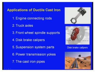
Now, these are the important applications of ductile cast iron. Engine connecting rods truck axles, front wheel spindle supports, disc brake calipers, suspension system parts power transmission yokes the cast iron pipes, and here we can see this is a connecting rod of in what say an internal combustion engine right.
