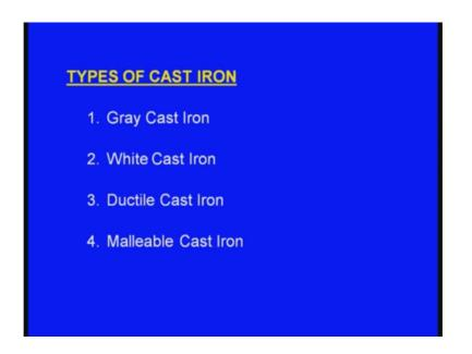
Now, there are mainly 4 types of cast irons. One is the gray cast iron. Second one is the white cast iron. Third one is the ductile cast iron. And the 4th one is the malleable cast iron.
