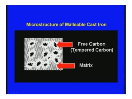
Now, we can see here again. So, this is this is the free carbon or the tempered carbon. Now again this is we can see the microstructure.
