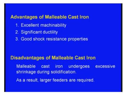
Next one it has got significant ductility. Next one good shock resistance properties. And these are the demerits or disadvantages of malleable cast iron. One is malleable cast iron undergoes excessive shrinkage during solidification. As a result, larger feeders or the risers are required.
