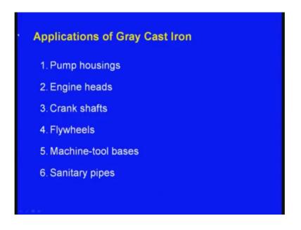
Now, these are the applications of gray cast iron. Pump housings, engine heads, crank shafts, fly wheels, machine tool bases, sanitary pipes. These are important applications in fact, there will be many more applications of gray cast iron.
