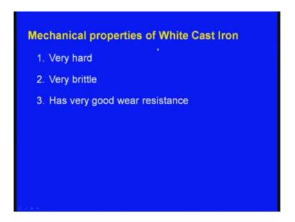
Now, these are the mechanical properties of white cast iron. Very hard why? Because cementite is present. Cementite is very hard, that is why the white cast iron is very hard. Next one it is very brittle, and it has got good wear resistance. White harder what say the cementite is very hard, because of that there is a good wear resistance.
