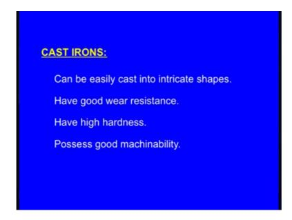
Now, cast irons can easily be cast into intricate shapes. We can make complex shaped castings. Next one they have good wear resistance. And they have high hardness and they possess good machinability. So, these are the important features and characteristics of cast iron.
