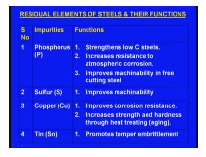
So, these are the residual elements. Phosphorus is present in the steels, right?
