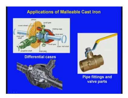
And here we can see few what say pictures. So, this is a differential oh in used in the automobiles. So, this is made up of malleable cast iron. Differential case and he this is the pipe fittings and valve parts. So, these are made up of malleable cast iron. Next one so far, we have completed the cast irons. Now let us see the cast steels.
