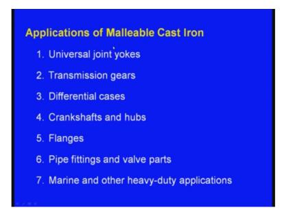
These are the applications of malleable cast iron. Universal joint yokes, transmission gears, differential cases crankshafts and hubs flanges, pipe fittings and valve parts marine and other heavy-duty applications. All these are made up of malleable cast iron.
