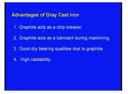
Now, these are the advantages of gray cast iron. Graphite acts as a chip breaker during machining. During the machining we require discontinuous chips. Because continuous chips would harm the tool as well as the surface finish of the job.
