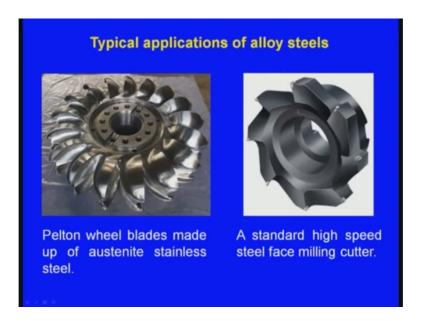
Now, we can see here these are the typical applications of alloy steels. So, this is a pelton wheel blades made up of austenite stainless steel. And here we can see this is a standard a high speed what say milling cutter made up of high speed steel. So, these are the applications of the alloy steels.
