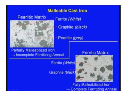
And again, we can see here we can see pearlitic matrix. And this is the this is the what the carbon packet. And again, here we can see this is the ferritic matrix, and this is the carbon packet or the graphite packet. And here it is partially malleable iron we can see and here we can see fully malleable iron.
