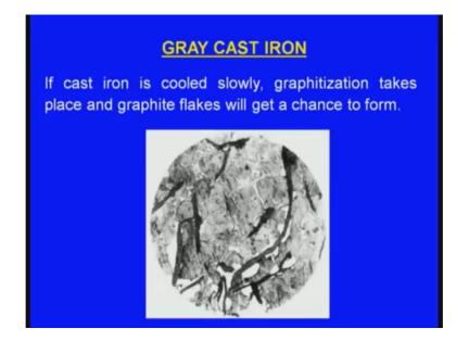
Now, this is the microstructure of gray cast iron. And we can see here these are all the graphite flakes. And several such flakes will be there all along the casting. So, this is the what say simple characteristic of the gray cast iron.
