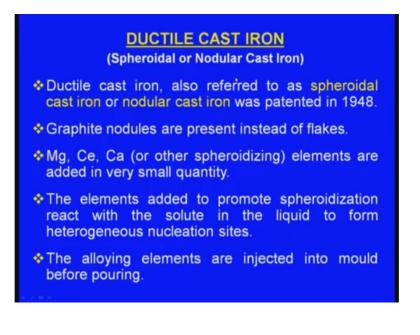
This brake shoe will be very good, it is condition will be very good. Next one let us see the ductile cast iron. What is the characteristic of ductile cast iron? Ducktail cast iron also referred to as spheroidal cast iron or nodular cast iron was patented in the year 1948. Now what is it is characteristic? Here in the case of the gray cast iron graphite flakes were present. And here graphite nodules are present instead of flakes. That is why we call it as the nodular cast iron.
