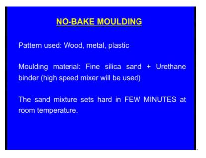
Our next process is the no-bake moulding. In the no-bake moulding the pattern used is the wood or metal or plastic and what is the moulding material? Fine silica sand and urethane binder. For this purpose, we need a high speed mixture and no hardener is required. Only thing is we need to mix the fine silica sand and urethane and pack around the pattern within few minutes the mixture will be hardened.
