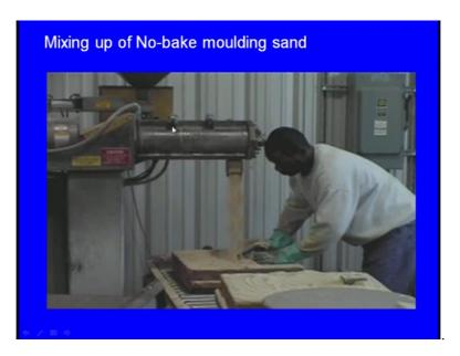
And here we can see this is the high speed mixture of the urethane binder and fine silica sand. As it now here we can see this is the pattern and this is the pattern is inside, this is
