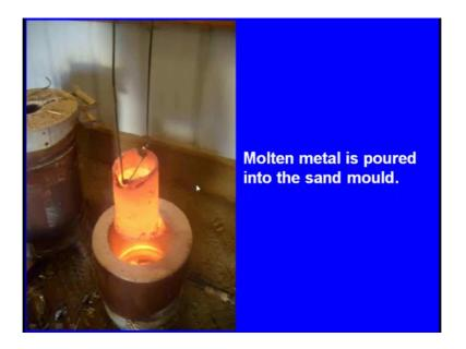
And here we can see the molten metal is ready for pouring.
