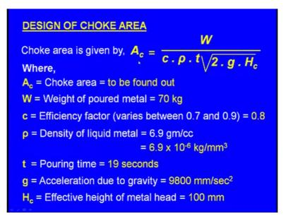
Now, in the previous lecture we have derived this expression for the choke area; choke area a c is equal to W divided by c rho t root of 2 g H c with A c is the choke area and in this case we have to find out W is weight of the poured metal, that is in this case it is equal to 70 kilograms c is the efficiency factor what is what is that because of the friction involved in the flow of the liquid metal.
