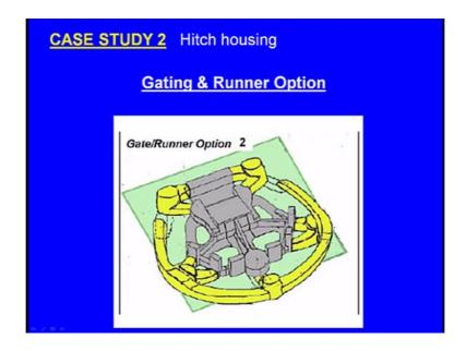
Now here is one ingate and here is one ingate likewise there are several ingates and the runner is surrounding the casting.
