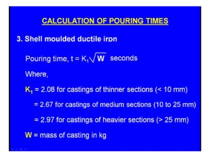
Now, how to calculate the pouring time; pouring times T is equal to K 1 root of W seconds, where K 1 is equal to 2.0 8 for castings of thinner sections or when the thickness is less than 10 millimeters. That is equal to 2.6 7 for castings of medium sections when the thickness is between 10 to 25 mm that is equal to 2.9 7 for castings of heavier sections when the thickness is more than 25 millimeters and W is the mass of the casting in kilograms.
