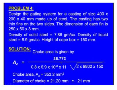
Now this is the choked area we are substituting different terms in the formula this is the weight of the poured metal and this is the what say c now this is the weight of the liquid density of the liquid metal and this is the pouring time.
