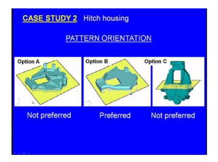
Now you see this option A the intricate shapes are facing upwards that be the case the molten metal may not exactly fill these shapes these intricate shapes that is why this is not preferred.
