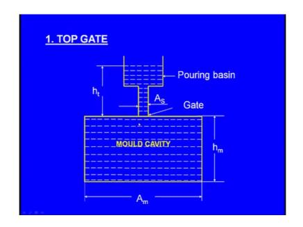
Now here we pour the molten metal through this way, initially the molten metal fills the pouring basin and it passes through this sprue and this is the choke and this is the also the gate then it enters into the mould cavity.
