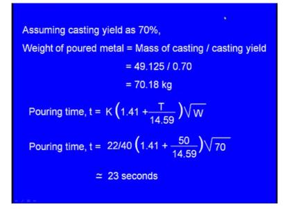
So, now, what is the casting yield casting yield means mass of the casting divided by mass of the poured metal multiplied by 100 usually we have seen that it varies from 70 to 80 percent
