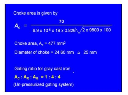
Now, choke area is given by A c is equal to 70 that is the weight of the poured metal 6.9 into 10 to the power of minus 6 into 19 this is the pouring time right and here, we have taken say 0.8 to 6 whole multiplied by 2 into 9800 into 100, choke area is equal to 400 and 77 square millimeters this is the what say choker area generally the choke area will be a circle that be the case what should be it is diameter.
