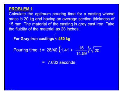
For gray iron castings when we what say pouring what say weight of the casting is less than 400 and 50 kilograms now problem 2 solve the previous problem if the material is steel.
