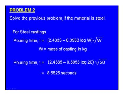
For steel castings pouring time T is equal to 2.4335 minus 0.3953 log W multiplied by root of W and here W is the weight of the casting.
