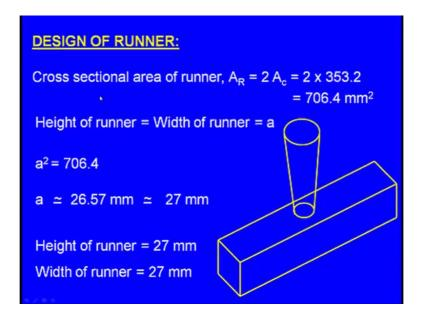
Design of the runner, now the cross sectional area of runner A R is equal to 2 into A C that is equal to 2 into 353.2 that is equal to 700 and 6.4 square millimeters. Now for your runner the cross section is a square, height of the runner will be equal to width of the runner let us assume that is equal to a, then a square that is the cross sectional area of the runner is equal to 700 and 6.4 and if we simplify this a is equal to 26.57 or it is 27 mm.
