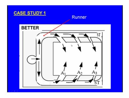
Now, the runner is like this the runner is surrounding the mould cavity you see this whole thing this is the what say sprue and this is the runner. The runner starts from here and it goes like this and it goes like this and up to here this is the runner again the runner is this side also it is like this. And here you can see this side there are 3 ingates here is one ingate, second ingate, and forth ingate and this side also one ingate second ingate and third ingates.
