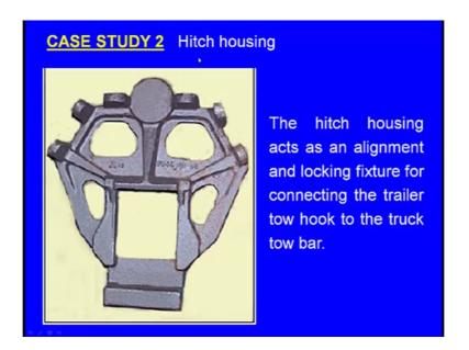
Let us consider a hitch housing the hitch housing acts as an alignment and locking fixture for connecting the trailer tow hook to the truck tau bar. So, this is the shape of the casting and how should be the what say pattern oriented inside the mould box how this runner should be designed. So, this is a again a case study let us analyze.
