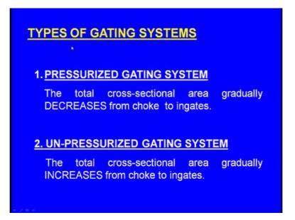
Now, one type is pressurized gating system and the second type is unpressurized gating system. In the pressurized gating system the total cross sectional area gradually decreases from choke to in gates now when we are pouring the molten metal. So, the molten metal enters into this sprue and it enters into the cavity at the choke sorry not at the cavity at the end the end of this sprue it passes through the choke.
