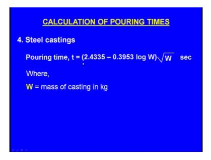
Pouring time T is equal to 2. 4335 minus 0.3953 log W multiplied by root W seconds where, W is mass of the casting in kilograms.
