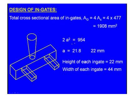
Now, this is the cross section of the ingate 2 a square is equal to 900 and 54 and if we simplify this a is equal to 21.8 that is almost equal to 22 millimeters.Now let us specify the dimensions of the cross section of the in each ingate, height of each ingate is equal to 22 millimeters width of each ingate will be equal to 44 millimeters.
