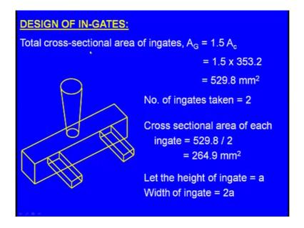
Now, the tot total cross sectional area of ingates A G is equal to 1.5 A C that is equal to 1.5 into 353.2 that is equal to 529 500and 29.8 square millimeters. Number of ingates here we are taking 2 now the cross sectional area of each ingate is equal to 500 and 29.2, they were 500 and 29.8 divided by 2 that is equal to 200 and 64.9 square millimeters and again the cross section of an ingate is a rectangle and the width of the cross section will be double then it is height.
