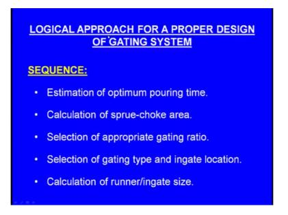
Now this is the logical approach what is this first one estimation of the optimum pouring time, second one calculation of the sprue choke area, next one selection of appropriate gating ratio, next one selection of gating type and ingate location, next one calculation of runner or ingate size. So, this is the sequence in the logical approach for a proper design of gating system.
