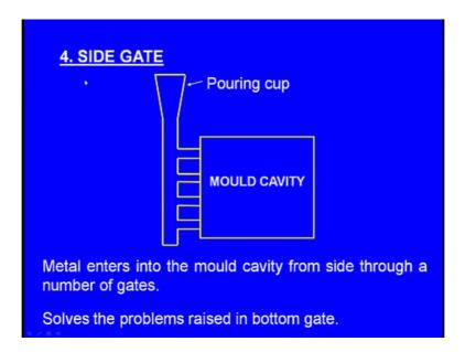
Next one the side gate, now you can see here this is the mould cavity and here the molten metal enters into the mould cavity along the sides on one side of the mould cavity we can see several in gates are there. Now this is the pouring cup and this is the sprue now the molten metal is poured here and the molten metal enters this way, it enters this way, enters this way finally, the whole cavity is filled with the molten metal.
