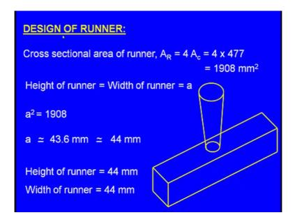
Now, next we need to find out the run design the runner what does it mean what is the cross sectional area of the runner, cross sectional area of the runner in the case of the unpressurized gating system A R is equal to 4 into A C that is equal to 4 into 400 and 77 that is equal to 1900 and 8 square millimeters.
