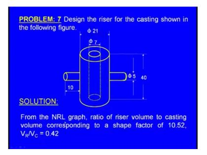
From the NRL graph ratio of riser volume to the casting volume corresponding to a shape factor of 10.52 that is V R by V C is equal to 0.42 that is what we have obtained from the graph.
