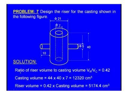
Now, ratio of the riser volume to casting volume V R by V C is equal to 0.42 casting volume. Say we have assumed that the casting is like a plate like a casting where the
