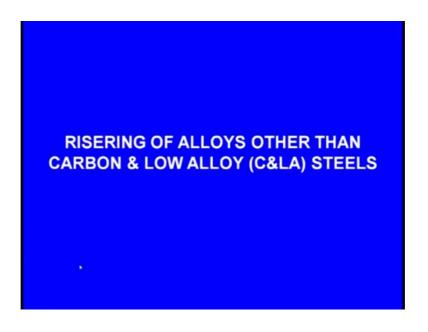
Now, risering of alloys other than carbon and low alloy steels in the beginning, I have told you that the NRL method or the naval research laboratory method which was a developed by HF Bishop and the team was applicable only for carbon and low alloy steels this cannot be applied for the other alloys.
