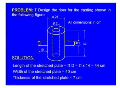
Now, we have another problem design the riser for the casting shown in the following figure. Now, what is this figure, what is this casting? This casting is a cylindrical casting and with an annular hole inside means, an axial hole is there parallel to the axis of the cylinder and the axis of the hole and the axis of the cylinder are coinciding. So, that is geometry of the casting.
