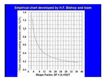
We can also find out the V R by V C ratio after that yes, there is a what say riser selection chart is there we can also find out the riser diameter and the riser height in different combinations.
