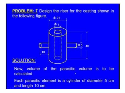
And we have to consider these parasitic elements until now we have assumed that these parasitic volumes are not there according we have assumed that the casting is cut and it is stretched.
