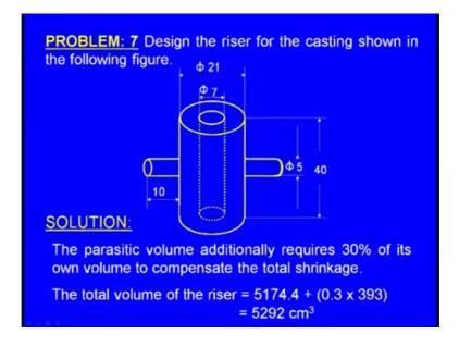
Now, the parasitic volume additionally requires 30 percent of its 1 volume to compensate the total shrinkage previously we have found out the riser volume that riser volume is enough provided these parasitic elements are not present, but once the parasitic elements are considered the volume of the riser must be more and what is the that excess volume in the riser that is the 30 percent of the volume of the parasitic elements.
