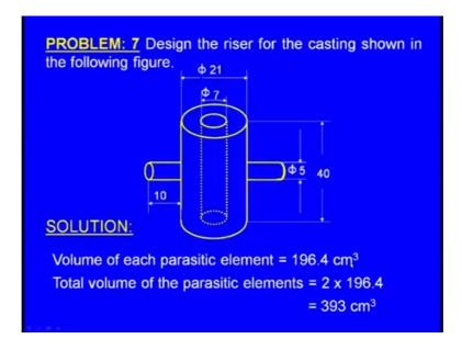
Total volume of the parasitic elements is just double 2 into 196 for that is equal to 393 cubic centimeters.
