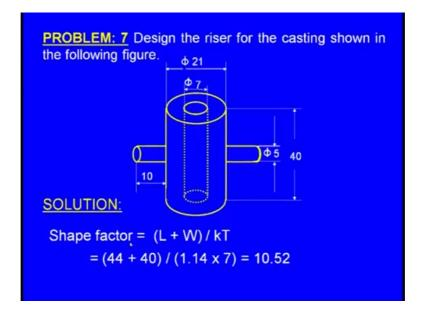
So, we have already seen length of that stretched plate. Imaginary stretched plate is 44 centimeters and the width is the same thing this much that is the 40 centimeters. All right and k is 1.14 and T is the 7 centimeters finally, we get your shape factor of 10.52.
