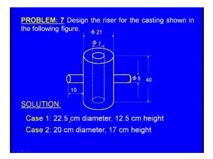
And in the one possibilities are in the first case the diameter of the riser is 22.5 centimeters and the height is 12.5 centimeters and in the second case or the second possibility the diameter of the riser is 20 centimeters and the height is 17 centimeters.
