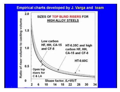
Now, this is the graph developed by the Varga and team. We can see here and only top blind risers for high alloy steels can be what say designed using these graphs and same shape factor is there on the x axis and what say V R by V C ratio is there on the y axis.
