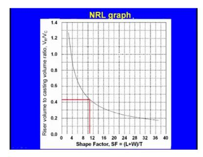
That graph is given by the steam, so this is that graph. In this graph the shape factor is plotted on the x axis and the riser volume to casting volume ratio V R by V C is plotted on the y axis. Once we could calculate the shape vector, from this shape factor we will draw a line then we will find out the corresponding V R by V R ratio. Then, we know the V C the volume of the casting. Then ultimately, we can know the volume of the riser required for the feeding of the required what say section.
