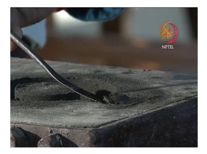
So, this is the gate cutter and there it should be limit inside the surface and this side we have the risering. So, we are linking a passes for the riser.
