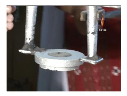
You can see this is the solidified casting and this is the casting this is the casting and this is the metal which is solidified in this sprue and this is the metal which is solidified in the riser. Later we have clean the casting and wing the cutting here. So, that these unwanted portions will be removed from the solidified casting.
