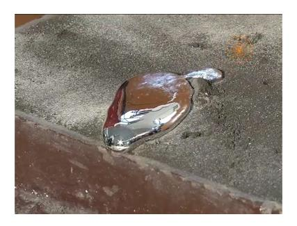
Hence now you can see most you can see withdraw poured molten metal through the pour for and it has drawn to this sprue and it has entered into the mould cavity then it has raise to the riser. So, this is the metal it has raised through the riser. So, that is how we
