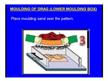
Now, after placing the sufficient moulding sand arrow above the pattern and inside the drag box now the sand has to be compacted. So, this is the rammer you see this is the hand rammer using the hand rammer manually it has to be rammed all over.
