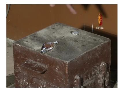
Now, I request Misses Saroj Sen Patnayak the research scholar and Mister Sukram the technical staff in our laboratory to carry out the shakeout operation. Shakeout operation means we have to break the sand and take the solidified casting outside. Now we will see the shakeout operation.
