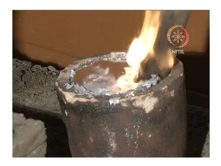
So, that is a graphite (Refer Time: 60:46) in which we can see the molten metal, that is the aluminium that is the aluminium. So, that is the pouring cup he is pouring through the pouring cup you see and it fills the cavity then it rises through the rise.
