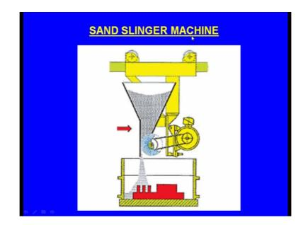
And here we can see the sand is here the moulding sand and there is a system which ensures that the sand will be falling above the pattern with a high pressure at a very high pressure.
