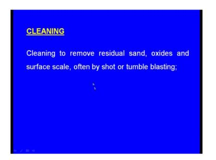
Next one the cleaning. After we do the knockout right after we give the heat treatment process the casting should be cleaned. So, this cleaning is to remove the residual sand though we have broken the sand taking the casting outside still some sand particles are attached to the casting. So, this residual sand particles are to be removed and some oxides will be there on the surface right some scales will be there and these are to be removed this is done by short or tumble blasting.
