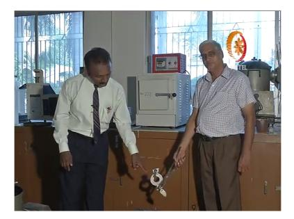
Friends now the shakeout operation is over we have broken the sand mould and we have taken the casting outside. So, this is the solidified casting you can see this is the actual casting, but this is the pattern which is solidified with the sprue core and this is the metal which is solidified with the riser. So, later these are the cut here, so that we will get the required casting.
