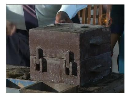
Next we will see the pouring of the molten metal into this mould.
