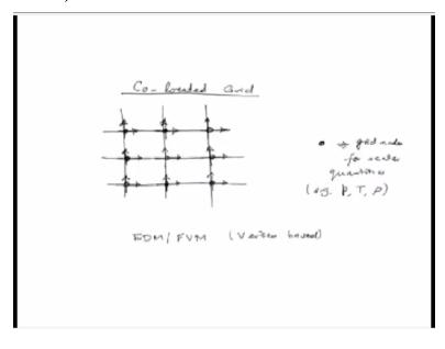
So first let us take a case of a structured grid which we might use in finite difference or finite volume formulations and suppose we take for instance, let us take vertex based grid, this is finite difference or finite volume grid vertex based. So let us use 2 symbols, we will use this field circles, field circles would represent the grid nodes for scalar quantities. For example, our pressure, temperature and density.
