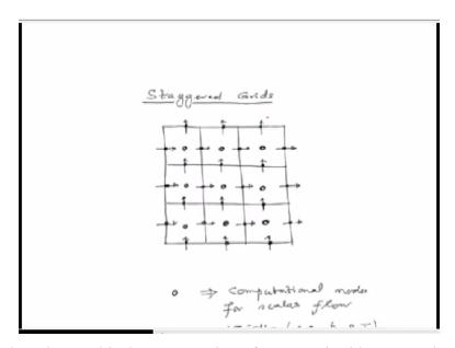
Let us have a look at the graphical representation of staggered grids. Let us draw for the sake of simplicity, a structured finite volume or finite and difference grid. Now the centroids are the ones where pressure or temperature would be defined, that is the way we are going to solve for all the scalar components. So our filled dots, they indicate computational nodes for scalar flow variables.
