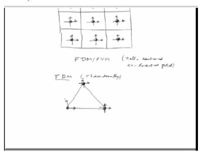
Similarly, if you are using cell-centred formulation that is our computational node is at the centre of a cell, so that is where all the other problem variables or flow variables are defined that is to say at the centroid, so field circles to represent scalar or similarly here. For velocity components also defined at these cell centroids. The situation is a bit more complicated in the case of finite elements, though theoretically this again our FDM or FVM cell centred co-located grid.
