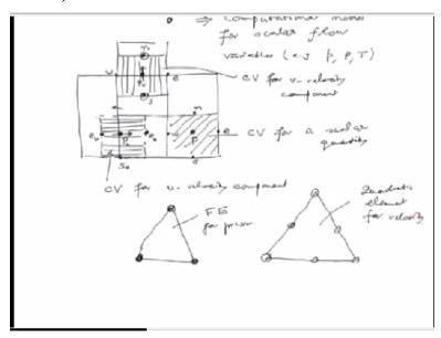
Now similarly if you are dealing with finite element, then you would use linear elements for pressure. This is FE for pressure and for velocity, we will have to use the quadratic element. This is quadratic element for velocity. The advantage I just mentioned.
