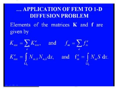
and matrices K and f, their elements were given by this Kmn=Sigma e Kmn for that particular element because we have taken the integral, we have summed it over the elemental integrals and so on and similarly, this fm is given by summing up all the terms corresponding to the load vector which we get from elements, so Sigma over e fme.
