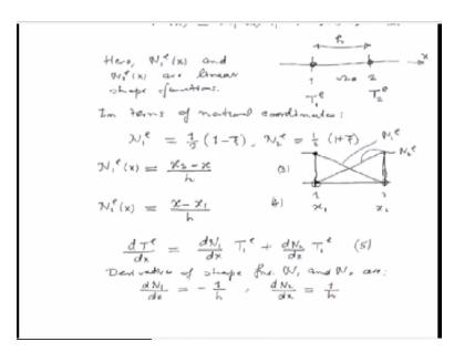
Value of the temperature at node 1, we will denote it by T1e, the value of the temperature at node 2 will be denoted by T2e. N1e and N2e are linear shape functions. So here N1ex and N2ex are linear shape functions. So if you want we can now use what we have learnt earlier in terms of the natural coordinates. So in terms of natural coordinates, what we have are N1e as given by  $1/2 \times 1 \times 1$  and N2 is given as  $1/2 \times 1 \times 1$ , okay.
