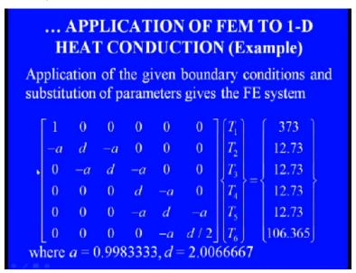
Let us say, remaining equations have been normalised a bit. First equation, you can clearly see, temperature is specified T1=373. So we have set the diagonal, this main diagonal term as 1. Remaining terms in this row as 0 and the right-hand side becomes 373 and so on, okay. Remaining terms that have been normalised, so that they appear close to the ordered 1, that is why we get this d is 2.00667 and of diagonal terms a take the value 0.9983333 and so on.
