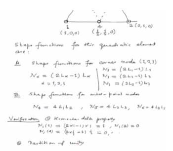
N alpha=2L alpha-1 times L alpha. So, alpha takes the values 1, 2 or 3. Let us demystify and write in expanded form. Let us write for each node separately. So, your shape functions N1=Twice of L1-1 times L1. N2=2L2-1 time L2 and N3=2L3-1 times L3. Now, can verify whether these satisfy the requirements which we had mandated for each shape function. Before we do that, let us write the shape functions for the remaining 3 nodes, i.e., midpoint nodes.
