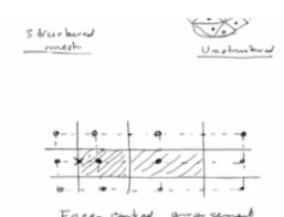
So, let us say this is our choice of the computational nodes and next what we do, draw the mid planes. For instance, between two for the time being, connect these with dotted lines. We need to find out the mid planes between these nodes which will define our control volumes surfaces. So, this is one of the mid plane, this is mid plane here. Similarly, mid plane between these two. So, these are the mid planes.
