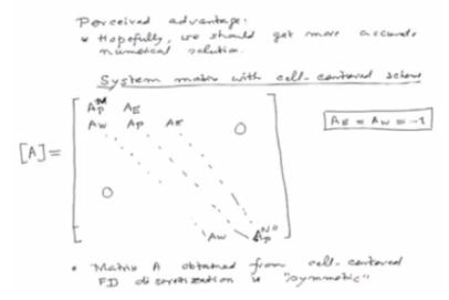
We use central difference scheme for the discretization of d2 T/ del x square term in our governing equation and we also used a central difference approximation for evaluation of dT/ dx term in the boundary condition, so what we said? Is; first thing is perceived advantages hopefully, we should get more accurate numerical solution either any other benefit, for that let us have closer look at the complete system when we assemble.
