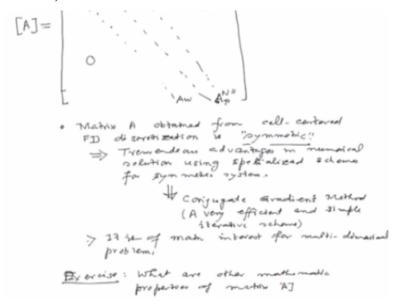
The first node was in the left boundary, the last node that is N+1 and that node was on the right boundary, there we saw that system matrix is not symmetric but here we have got a symmetric system matrix which has got scores of advantages in numerical solution okay. So we have got tremendous advantages in numerical solution because we have got specialized schemes for symmetric systems, using specialized schemes for symmetric systems.
