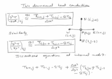
Two dimensional heat conduction and what we are doing the way, we are proceeding now that can be easily extended to 3 dimensional problems, so 5 point CDS molecule we are just dealing with the stencil, so these nodes could be at the cell centre, so that these could be at the edges, we do not need really need to worry about it, so our node P ij system neighbour Ei+1, j western neighbour Wi-1,j its northern neighbour in y direction, it will be ij+1.
