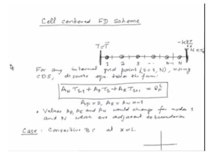
Cell centered finite difference scheme, let us draw our grid, our nodes are located at this centroids of each of these cells node 1, 2, 3 and so on, N-1 and N, this is our right boundary where we have a conductive boundary condition specified and we had at left boundary T = T bar, here we have -k del T/ del x = H \* T - Ta, so they mentioned earlier as for; since all these grid points happen to be internal.
