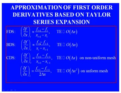
So we derived a forward difference approximation del f/del x at point i=f of i+1-fi/xi+1-xi which is stands for delta xi and truncation error is of the order of delta x, backward difference scheme by using values at the point left towards current point so del f/del x at point I approximately=fi-fi-1/xi-xi-1truncation error is still of the order x. So both of these schemes are first order accurate.
