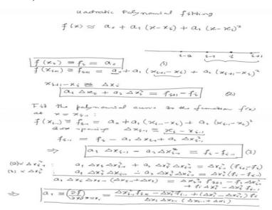
We want to have a quadratic polynomial fitting, so f of x that is would be approximate by the polynomial a0+ a2 times x-xi+ a2 times x-xi whole square, so here we have got 3 unknown coefficients a0, a1 and a2 and these we would determine by using function values at point i, i-1 and i-2 or rather let us take a centralized difference formula, let us use the values at i, i-1 and i+1. So they are 3 node points.
