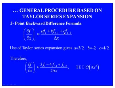
So one simple example of this 3 point backward difference formula that if you want to use values at to downstream nodes or backward nodes, in addition to the function value at point xi so afi+bfi-1+cfi-2/delta x this would give us difference approximation to the first order derivative at del f/del x i. Now let us try and get the values of these coefficients by performing a simple Taylor series expansion.
