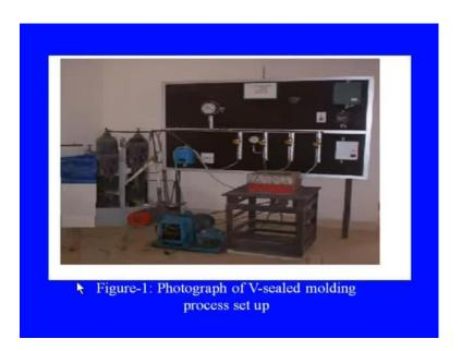
Here is the setup in your screen. So, here this is the vacuum pump which creates vacuum and this is connected to, this is the mold system where the vacuum connections are there and the table is given vibration through this motor arrangement.
