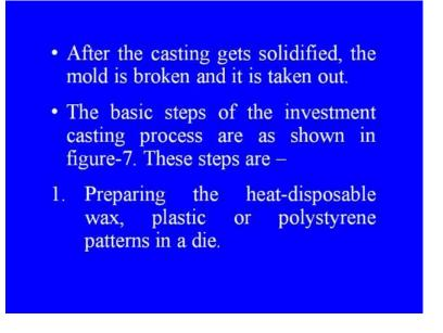
After the casting get solidified the mold is broken and it is taken out. The basic steps of the investment casting process are as shown in the figure seven. These steps are number one preparing the heat disposable wax, plastic or polystyrene patterns in a die.
