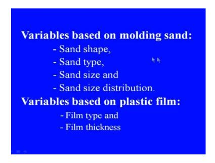
The variables based on molding sand, sand type, sand shape, sand size and sand size distribution. Then another group is variables based on plastic film in which film type and film thicknesses are of major concern. Next group is variables based on vibration in which amplitude and frequency of vibration apart from the time of vibration are of major concern.
