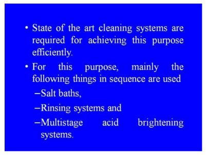
State of the art cleaning systems are required for achieving this purpose efficiently. For this purpose mainly the following things in sequence are used. Number one salt baths which will be able to remove most of the things from the body, then rinsing systems which will further remove those which are still sticking, then multistage acid brightening systems. If there are any further the acid will remove them with their reactive nature.
