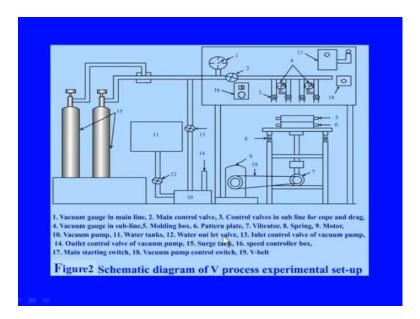
This can be further seen in this setup, schematic diagram, this is what the vacuum pump I was talking about in the previous photograph and then this is the vibratory system which shakes the table which is mounted on this spring mounted table. And this is the mold mold box, these are the connections for the vacuum which is connected through this and
