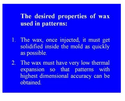
The number two, the wax must have very low thermal expansion so that patterns with highest dimensional accuracy can be obtained. This is another very important aspect as far as the accuracy of the product are concerned. The product accuracy will depend to a large extent to the accuracy of the pattern and pattern on the other hand will depend, the accuracy of the pattern will depend on the material of the pattern. Therefore, the wax we
