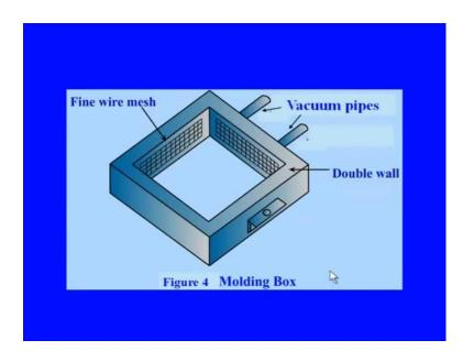
This is the molding box. A typical figure used in this process. This is the double wall box and this is the fine wire mesh system. The pattern, the patterns used in vacuum process are similar to the pattern used in other conventional sand casting processes. Numerous small holes are created on the vertical edges of the pattern used in the V process. Hence, the plastic film correctly adheres to the vertical surface of the pattern thus creating the right cavity in the mould.
