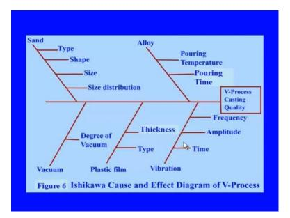
Here is the Ishikawa cause and effect diagram. These are the major parameters like sand. In sand the type of sand, shape of the sand, size of the sand and size distribution of the sand causes or can cause some quality best product parameters in this process. Then the other parameter is the alloy based parameters. Here the pouring temperature and the pouring time are the main parameters that can affect the quality of the product.
