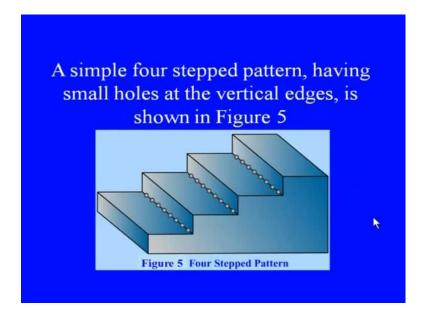
A simple four stepped pattern having small holes at the vertical edges is shown in this figure. These are the small holes and this is the four stepped pattern, the vacuum system. Vacuum is applied to the molding box containing sand to (()) the mould as well as to withdraw the decomposed gases. It remains constant and active during pouring of molten metal till solidification.
