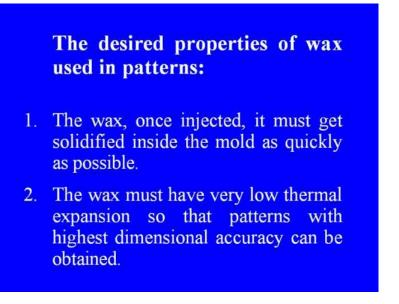
Number one, the wax once injected it must get solidified inside the mold as quickly as possible. So, longer the time to take, get solidified lower will be the productivity.
