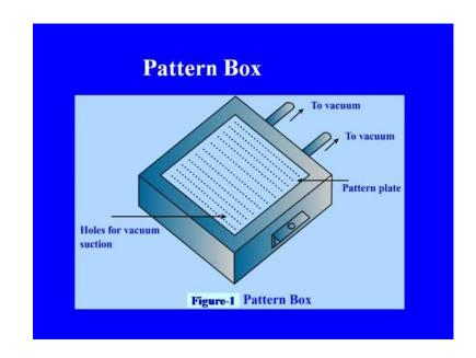
This is the figure of a pattern box, these are the small holes for suction for vacuum, this is the pattern vacuum pattern plate and this is the arrangement for the connection to the vacuum system.
