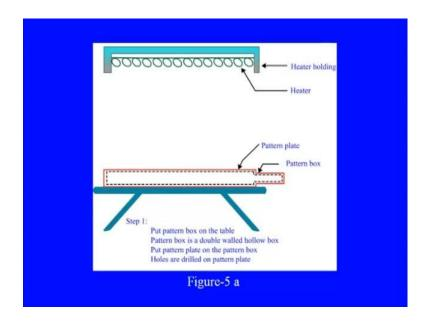
The first step is as shown in the screen here, the pattern box on the table is placed like this, then the pattern plate is places on top of the pattern box.
