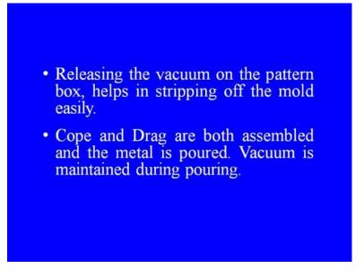
Releasing the vacuum on the pattern helps in stripping off the mold easily. Cope and drug are both assembled and the metal is poured vacuum is maintained during pouring. The vacuum is further released once the mold box is cooled, this allows sand to freely flow back there, by leaving a clean casting behind the sequence of producing the casting made by vacuum sealed molding process, is shown in the following figures.
