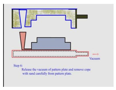
Now, the vacuum is released and this is removed from the pattern plate, then prepare the drag in the same way.
