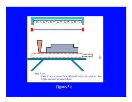
In the next step, the heater is switched on this heats the film and put it over the pattern plate. Then simultaneously, vacuum is also applied to the pattern box.
