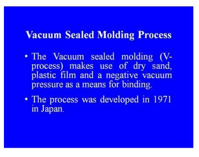
The vacuum sealed molding process also known as V process makes use of dry sand plastic film and a negative vacuum pressure as a means for binding. The process was developed in 1971 in Japan thus this can be regarded as a young process in the family of casting due to its unique capability in producing smooth and accurate castings. The process gained further importance the basic difference; that exists between the V process
