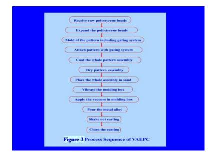
This is the complete flow chart of the vacuum assisted evaporative pattern casting process. The first thing in the first stage raw polystyrene beads are received. They are expanded, then the mold of the pattern including the gating system is been made. Then
