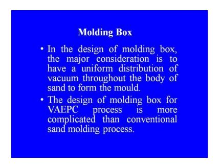
The molding box, in the design of molding box, the major consideration is to have a uniform distribution of vacuum throughout the body of sand to form the mold .The design of molding box for VAEPC process is more complicated than conventional sand molding process. The box has to be made, which annular wall on all the four sides inside
