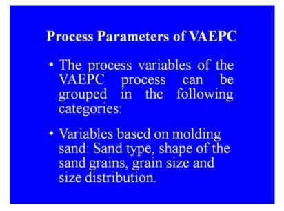
Now, let us see the process parameters, that affected the vacuum assisted evaporative pattern casting. The process variables of the vacuum assisted evaporative pattern casting process can be grouped in the following categories. Number one, the variables based on molding sand, these variables are sand type shape of the grand sand grains, grain size and size distribution.
