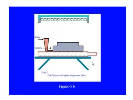
In the next step with sprue is placed on the pattern plate, this is the sprue and this is the pattern.
