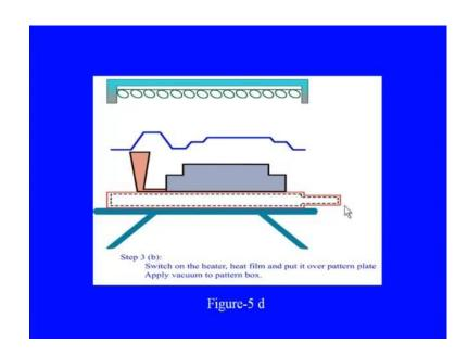
In the next step, the heater is switched on the film is heated and it is put over the pattern plate. Then vacuum is maintained in this step the vacuum is maintained on the pattern box.
