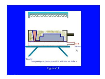
In the next step, the cope is put on the pattern plate and it is with sands and it is shacked.
