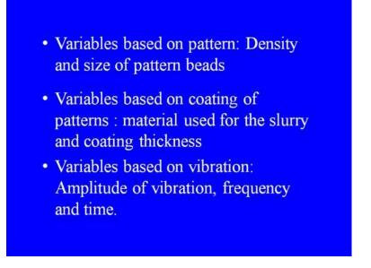
Number two, variables based on pattern, these variables are density and size of pattern beads. Number three, variables based on coating of patterns, variables are material used for the slurry and the coating thickness. The number four groups of variables based on vibration, here the variables are amplitude of vibration. Vibration frequency and time the next group of variables are based on vacuum.
