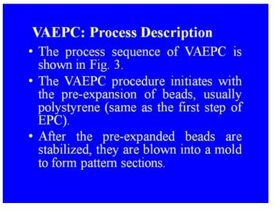
The procedure initiates with the pre expansion of the beads usually polystyrene. This is same as the first step of the earlier discussed evaporative pattern casting process. After the pre expanded beads are stabilised, they are blown in to a mold to form pattern sections.
